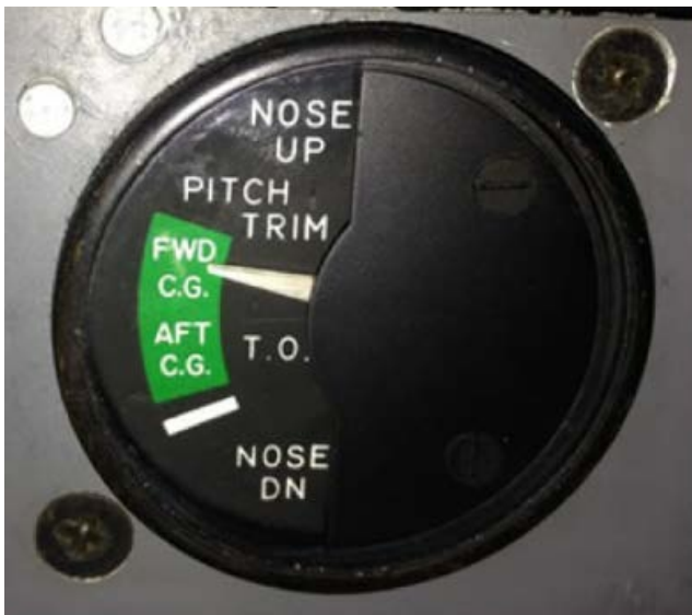
Figure 1: Cockpit indication with horizontal stabiliser in the neutral (take-off) position
