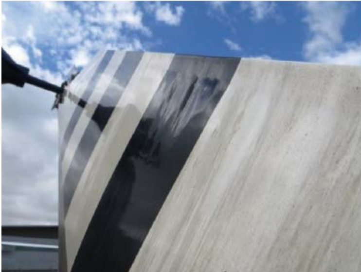
Figure 1: Damage to ESD tail rotor
