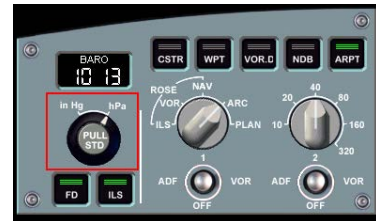
A320 EFIS control panel
