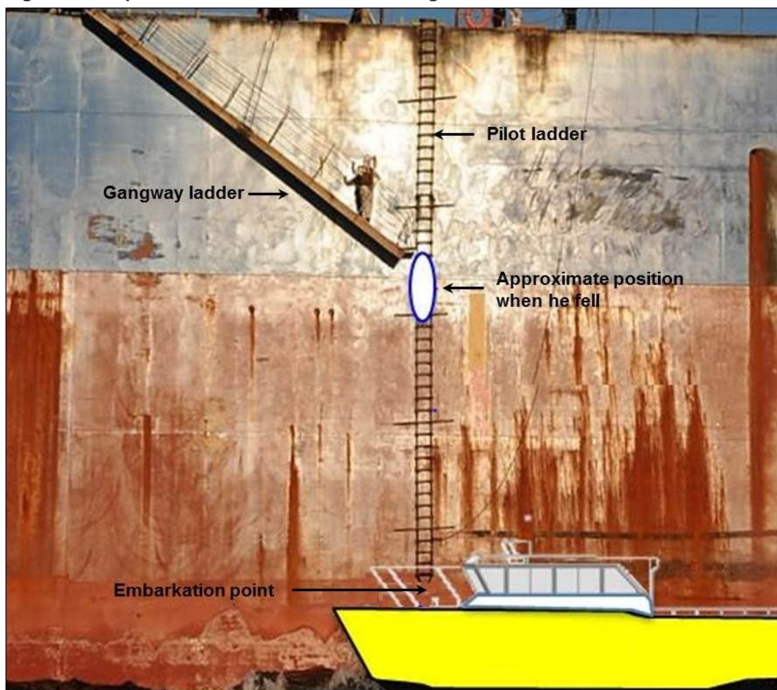
Figure 3: The port side combination ladder arrangement
