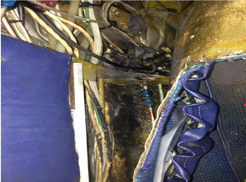
Figure 1: Fire damage behind the left internal panel of VH-SBS
