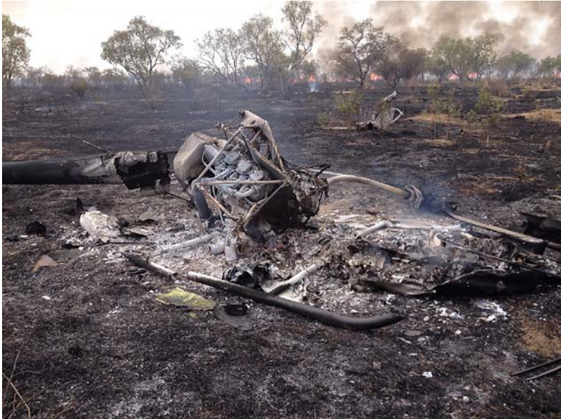
Figure 1: Fire damage to VH-TZE and surrounding bush
