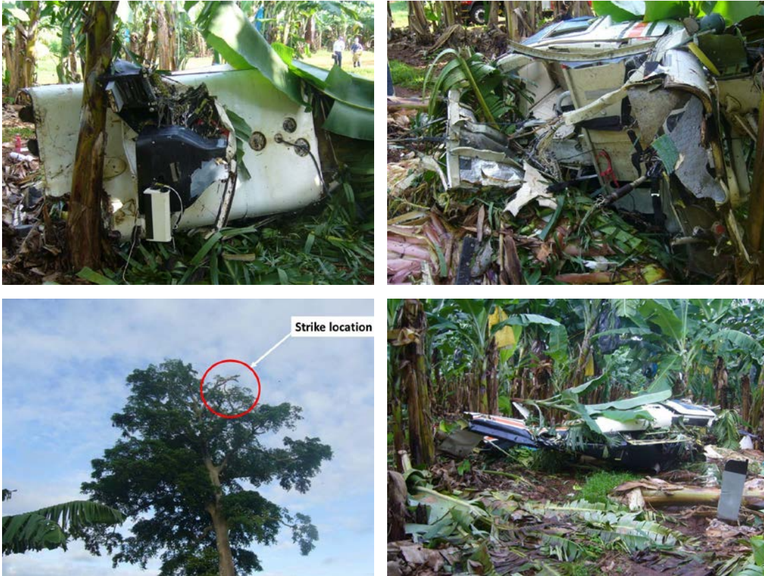
Figure 1: Damage to VH-BNG and large tree strike
