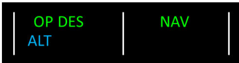
Figure 5: Representation of FMA vertical and lateral modes before and after the approach mode was selected (APPR push-button pressed)
