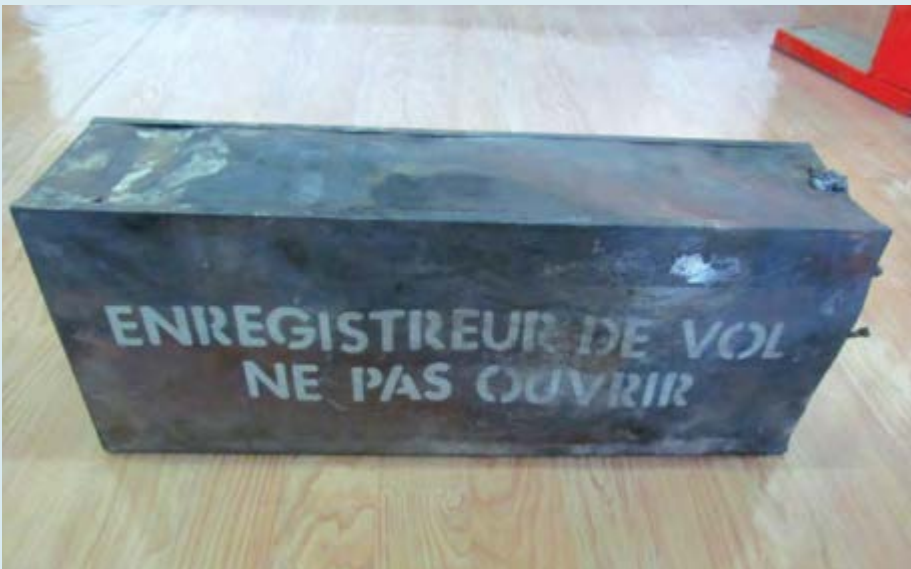
Severely fire-damaged flight data recorder—as received
