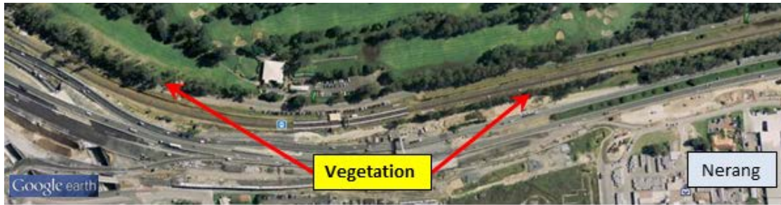
Figure 20: Railway station locations recording a high incidence of train overruns where trackside vegetation on the approaches was identified.
