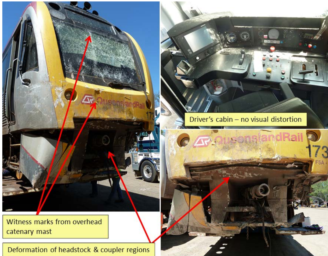
Figure 15: Resultant damage to the front of car 5173 after colliding with buffer stop, overhead electrical catenary mast and station building.
