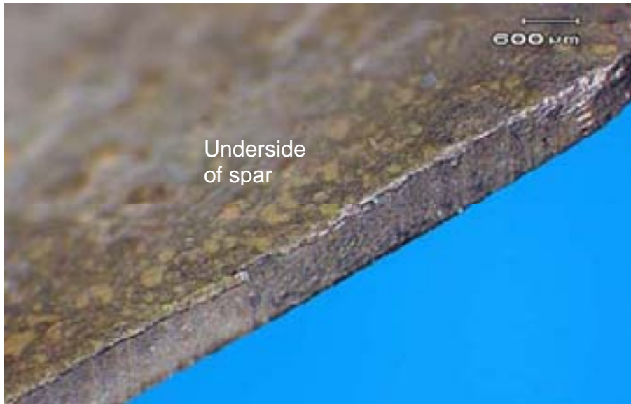
a) VH-OHA, s/n 6249A, fractured blade, showing a sharp corner between the spar end and the bonded surface, and, in addition, minimal surface roughening by grit blasting
