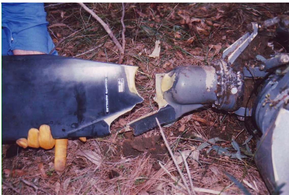
Figure 2: Failed 'blue' main rotor blade
