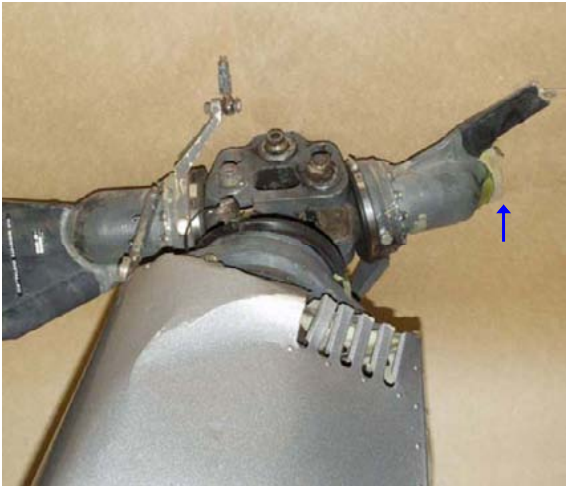
Figure 1: The recovered main rotor head assembly, VH-OHA
