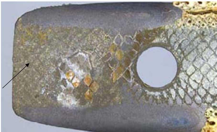
b) VH-OHA intact blade, adhesive bonded to the spar, at the spar end is arrowed
