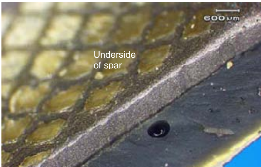
b) Blade s/n 8603B, showing a rounded corner between the spar end and bonded surface, plus surface roughening by grit blasting
