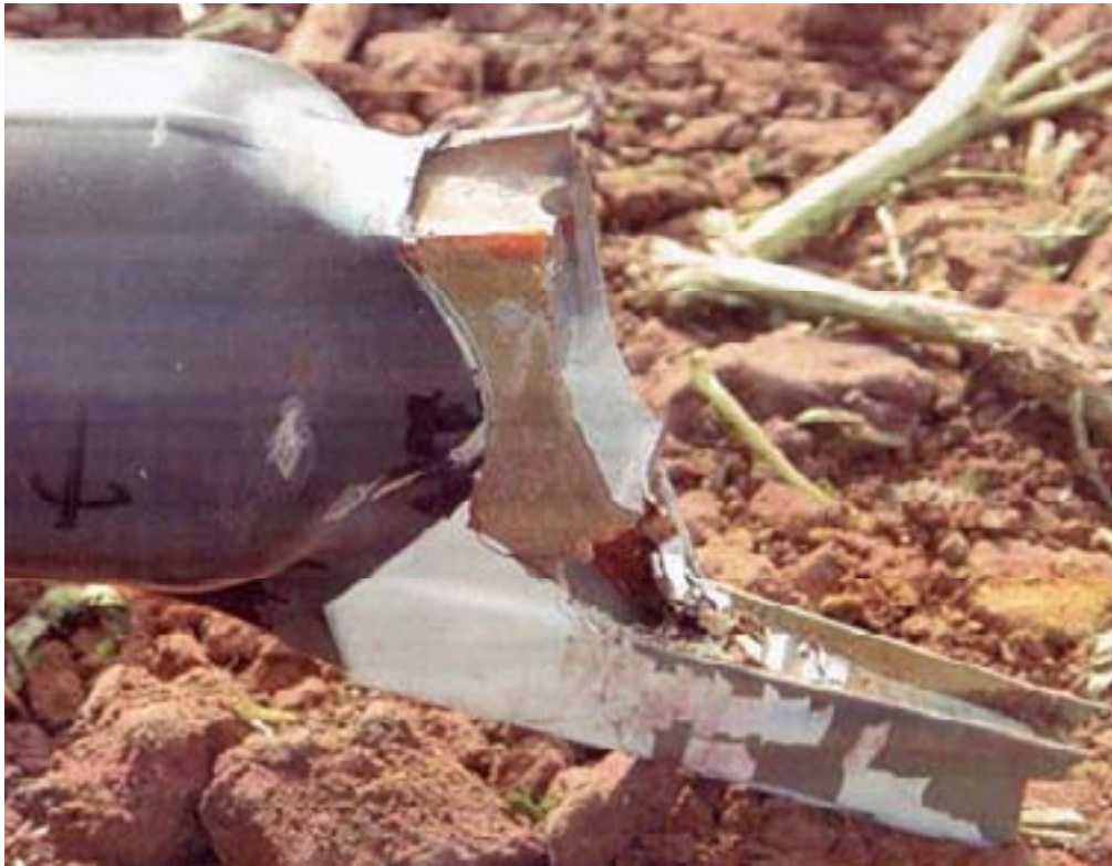
c) The root fitting side of the fracture, as recovered
