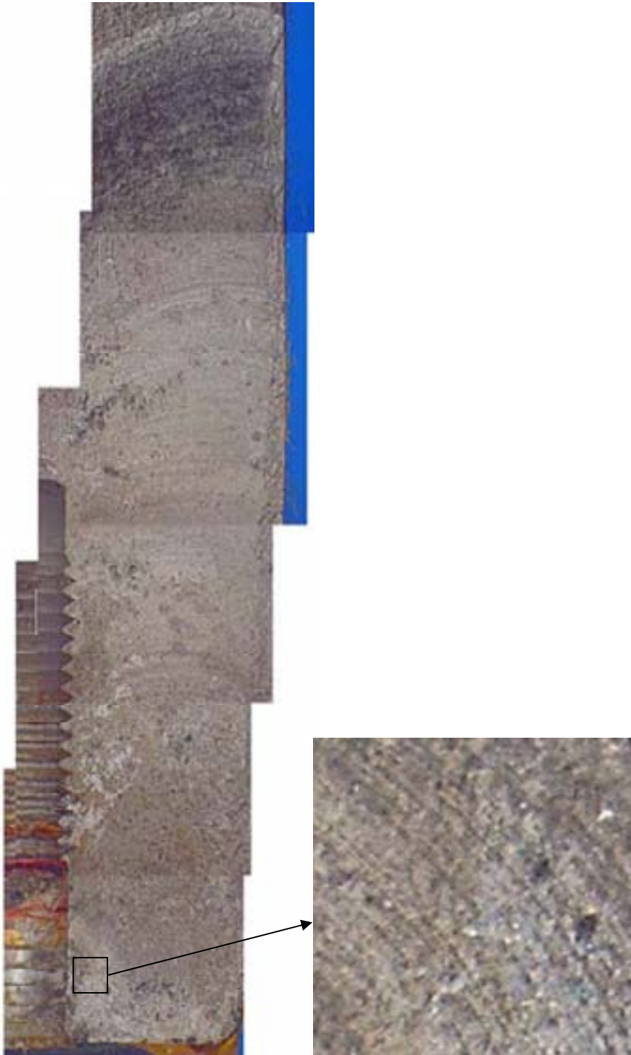
Figure 10: Photomontage of the fatigue fracture (lower half)
