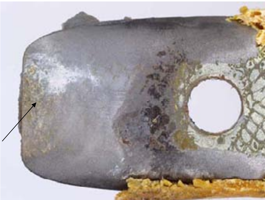
b) VH-LDR intact blade, adhesive bonded to the spar, at the spar end is arrowed
