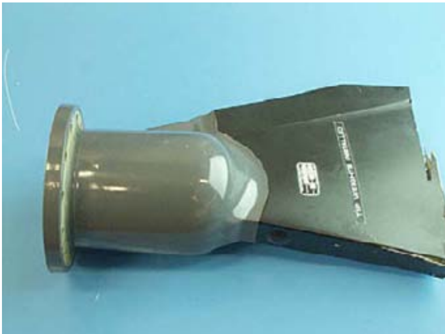
Figure 1. General condition of blade root end, upper and lower blade surfaces.
