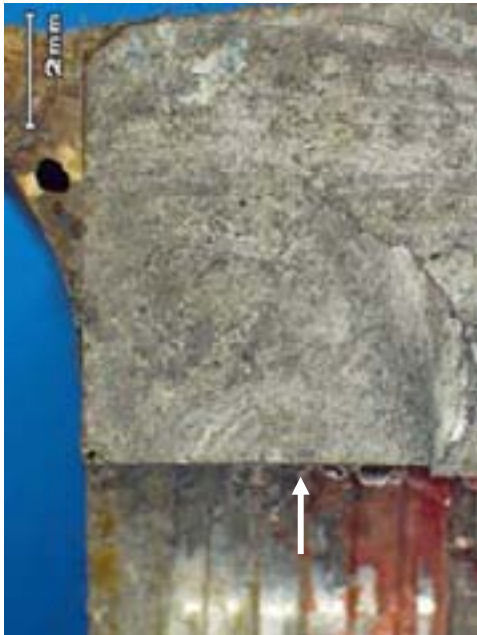
a) Third initiation site, crack growth from this site was influenced by the presence of the crack growing from second initiation site
