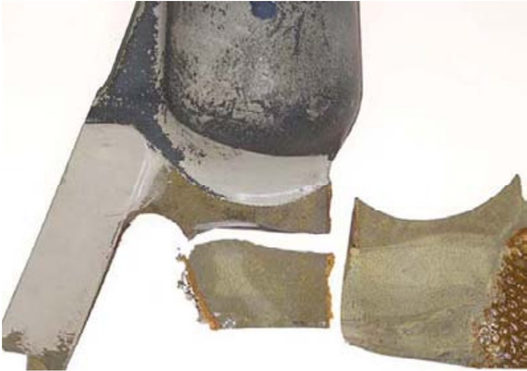
a) Disbonding extends from the inboard edge of the skin to the fracture. The paint film on the root fitting was badly weathered
