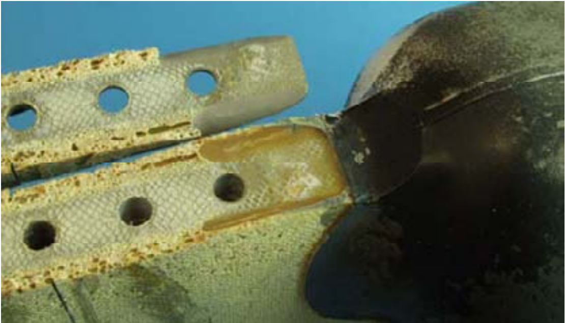
a) Disbonding has extended from the end of the spar to the edge of the inboard bolthole
