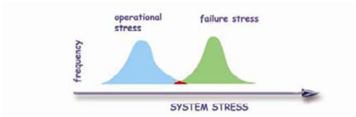
Figure 19: Schematic illustration of the probability of failure under conditions of variable operational stress and failure stress - failure condition
