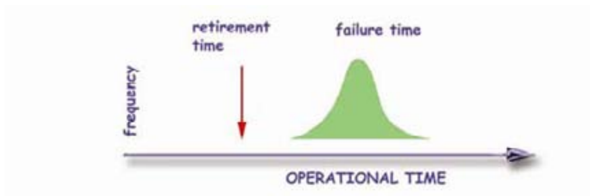
Figure 16: The desired relationship between retirement time and failure time
