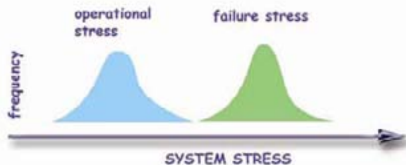
Figure 18: Schematic illustration of the probability of failure under conditions of variable operational stress and failure stress – no failure condition
