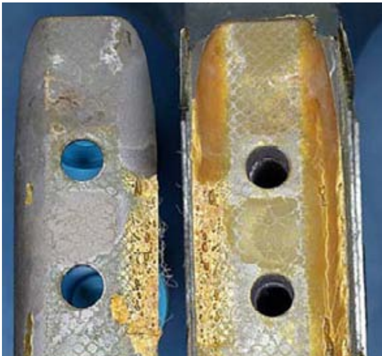
b) VH-LOT, s/n 8414B. Extensive disbonding has occurred, including disbonding between the two boltholes. However disbonding has not extended to the edge of the inboard bolthole.
