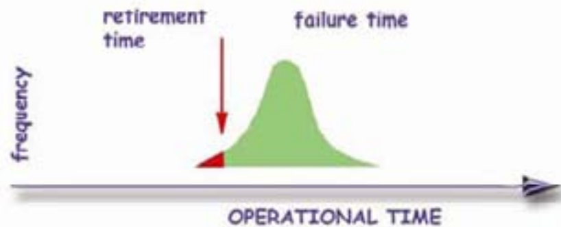
Figure 17: The relationship between retirement time and failure time that results in the failure of a number of components of a particular configuration
