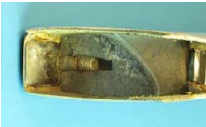
b) The blade side, or outboard side, of the fracture
