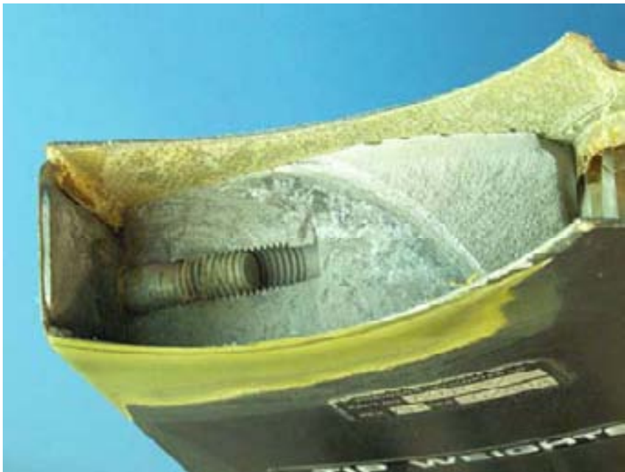
b) Looking up from the lower surface of the blade
