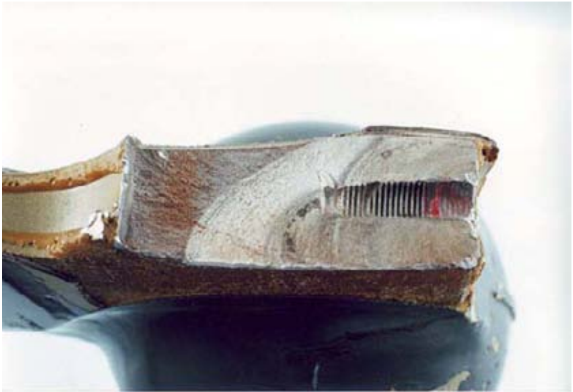
d) The root fitting side of the fracture, as recovered
