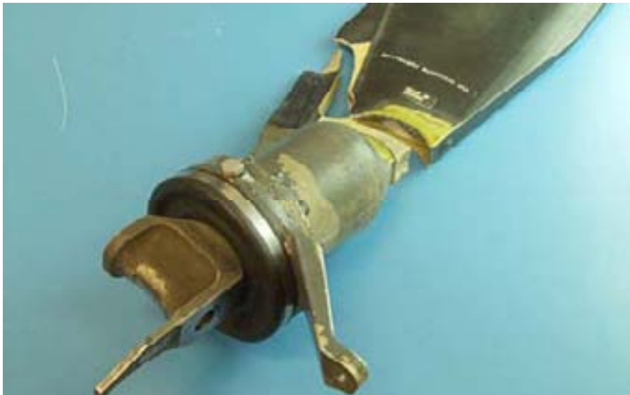
Figure 2: The fractured main rotor blade, VH-OHA
