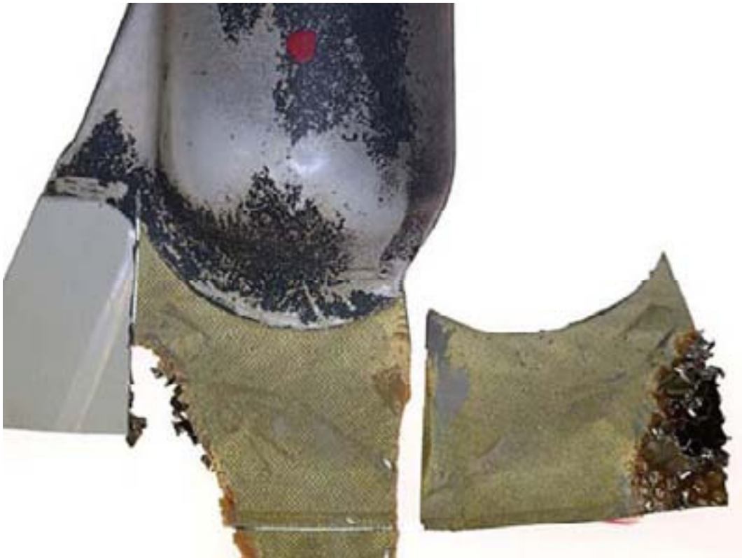
Figure 15: The nature of the adhesive bond between the upper and lower blade skins, blade s/n 6283A
