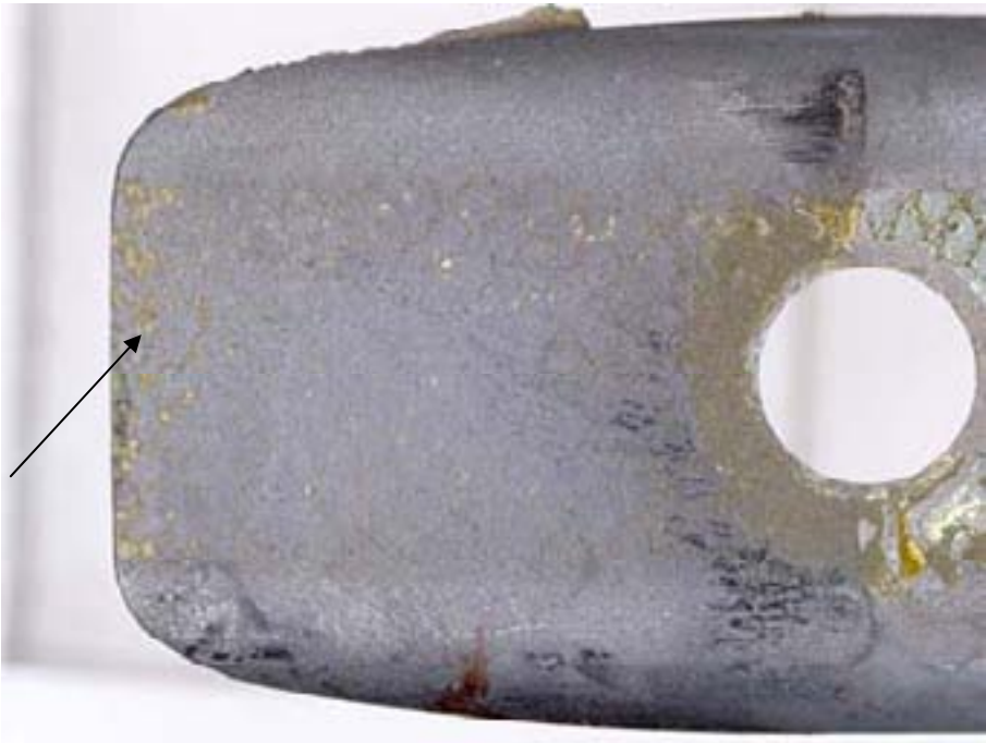
a) VH-LDR fractured blade, adhesive bonded to the spar, at the spar end is arrowed
