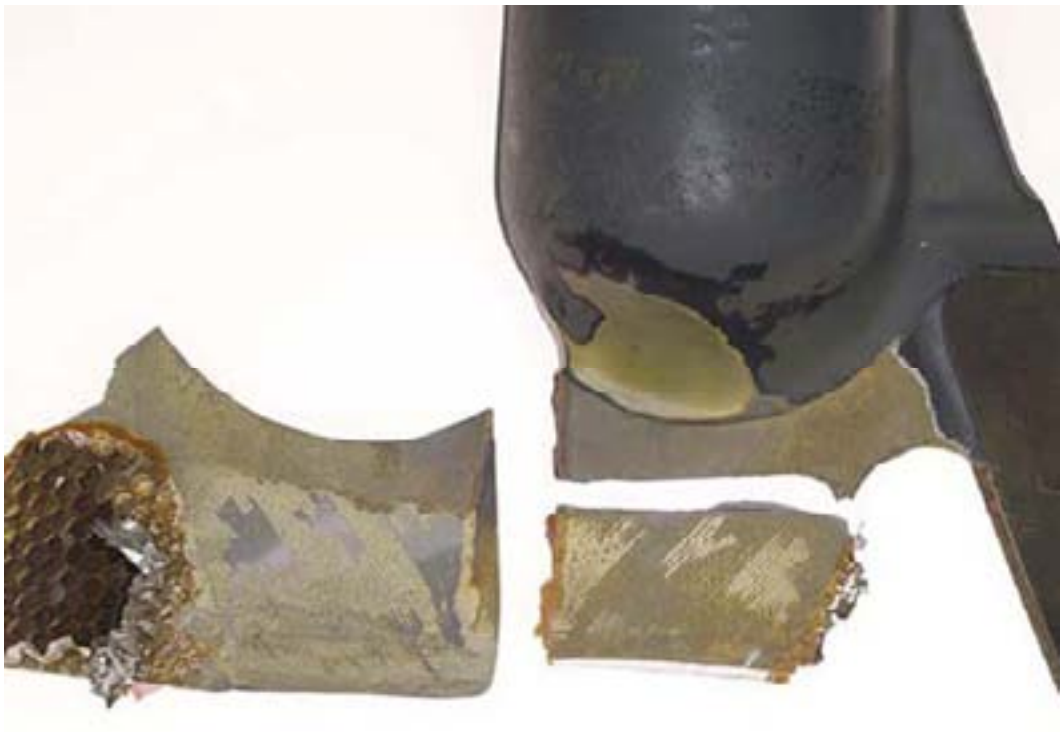
b) Disbonding extends from the inboard edge of the skin to the fracture
