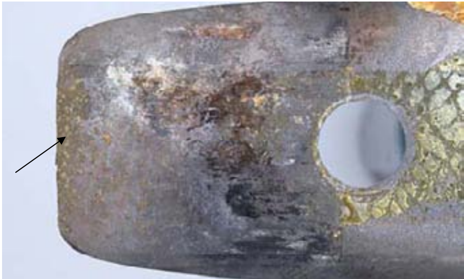
a) VH-OHA fractured blade, adhesive bonded to the spar, at the spar end is arrowed
