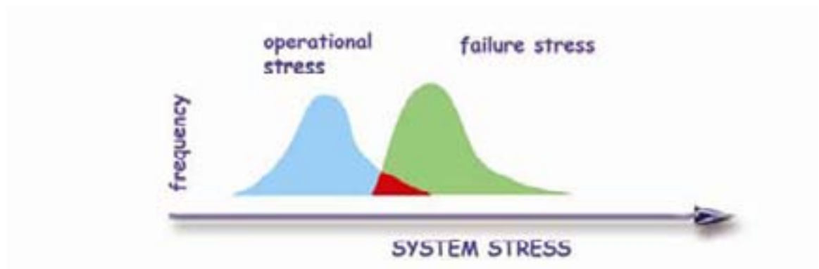
Figure 20: Schematic illustration of the probability of failure under conditions of variable operational stress and failure stress, failure condition – the effect of skewed distribution
