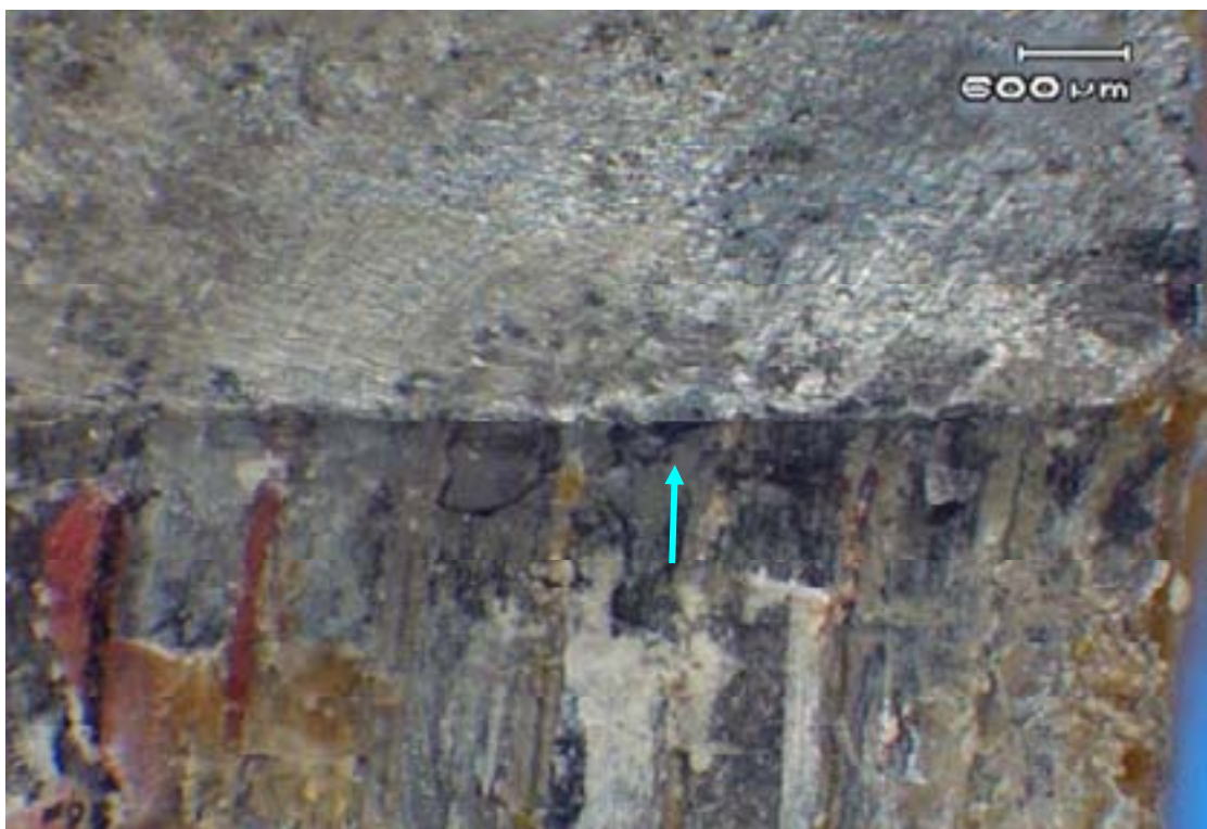
Figure 9: Extended focus light microscope image of the first initiation site
