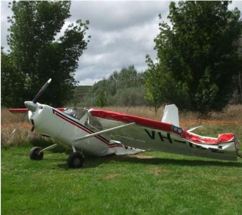
Figure 2: VH-ICE damage to the left wing
