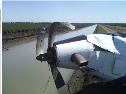
Power line wrapped around propeller
