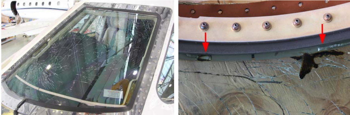
Figure 1: Shattered left windshield external (left) and internal (right)
