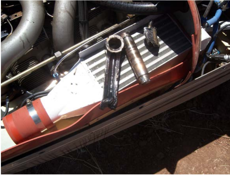
Figure 3: Engine number two cylinder failed parts
