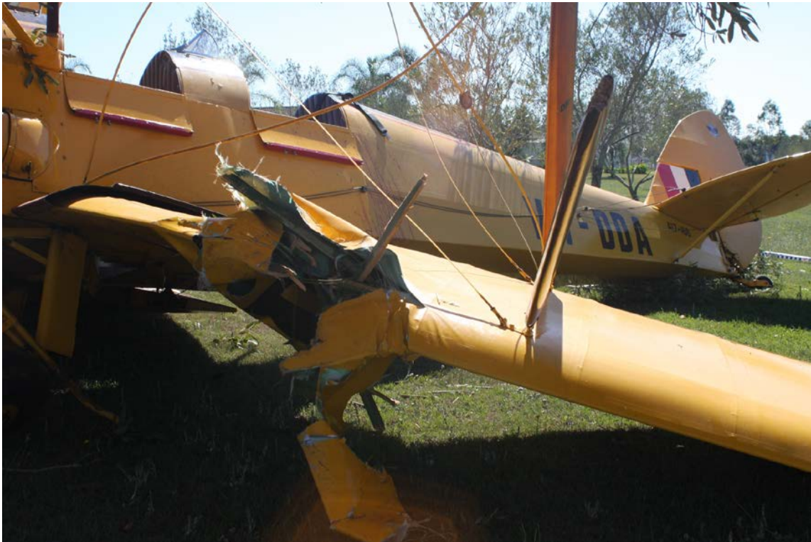
Figure 1: Damage to left wing following impact with a tree
