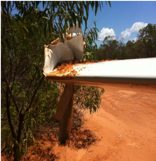
Figure 1: Right wing and nose gear damage
