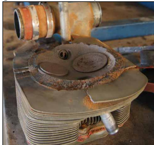
Figure 3: Failed number-4 cylinder
