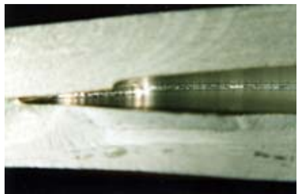
Fig. 44. Edges of the internal cavity, showing a continuous fillet of a metallic alloy.
