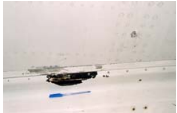
Figs. 34 (Left) & 35 (Right). Impact damage found on the fuselage and trim panels at station 1140, above the wing root.
