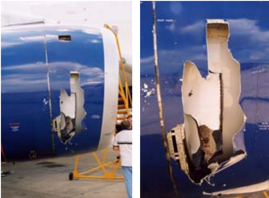
Figs. 18 & 19. External damage to the right side of the intake cowl.
