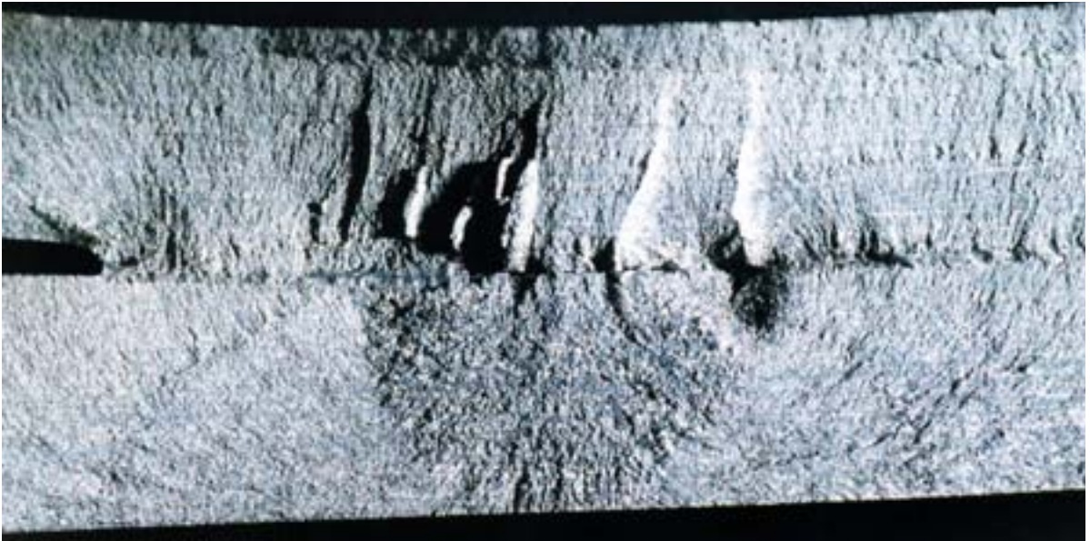
Fig. 45. Obliquely lit view of the blade fracture surface, centred over the fatigue initiation site. Note the thumb-nail-shaped area of initial crack propagation to the external (convex) surface.
