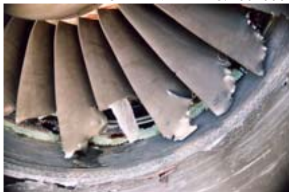
Fig. 4. Damage sustained by the fan blades – many had fractured through the internal cavity.
