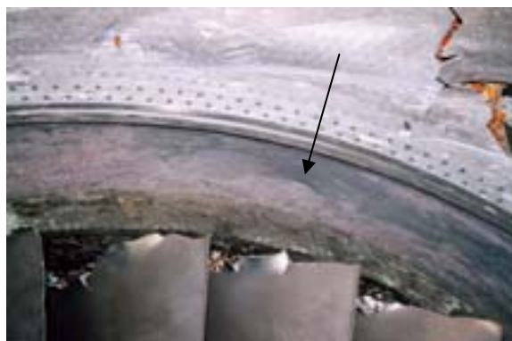
Fig. 6. Closer view of the blade primary impact point. Alignment with the blade pitch angle can be seen.
