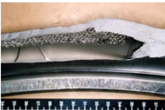
Fig. 43. Inside surfaces of the exposed blade cavity, showing remnants of the internal honeycomb material.
