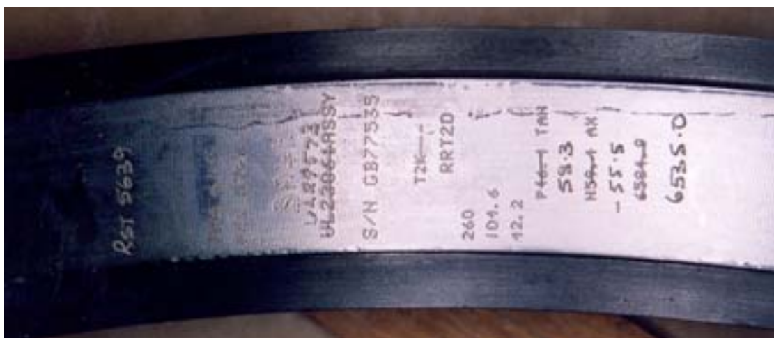
Fig. 42. Identification engraved / stamped on the underside of the failed blade.
