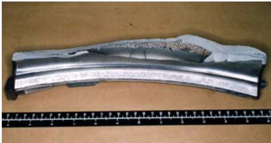
Fig. 41. Stub of the fractured blade after general laboratory cleaning. Leading edge is to the left.
