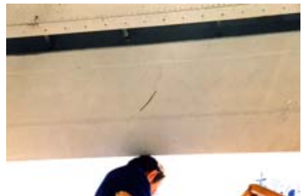
Fig. 32. Deep scoring to the undersurface of the aft trailing edge flap.
