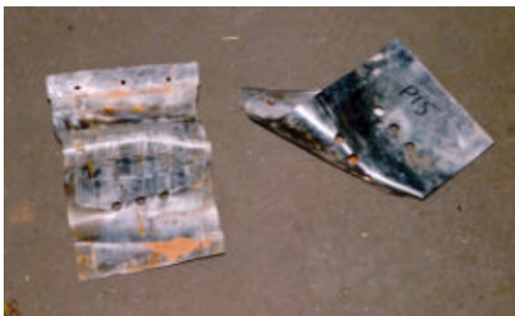
Fig. 8 (top L). Debris and remnants of the HyShot scramjet payload and Orion motor casing.
