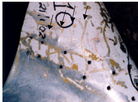
Fig. 52. Nike fin skin section showing a clear impact mark from the leading or trailing edge of another Nike fin. Note the row of rivet indentations.
