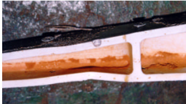
Fig. 53 (left). Clamping point for the fin securing lug – note the disruption produced by in-flight movement.
