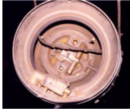
Fig. 36. Internals of the adapter unit, showing the ignition mechanism. All surfaces were free from combustion products.
