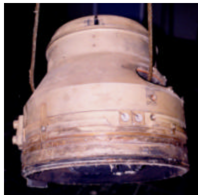
Fig. 34 (right). Opposite side of adaptor – damage free.
