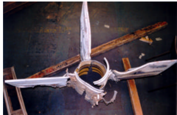
Fig. 14. Re-assembled sections of the tail can, showing the orientation and positions of the recovered fins.
