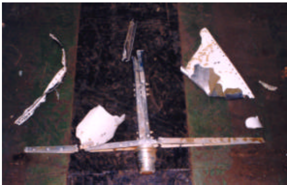
Figs. 47, 48 (top left & right), Figs 49, 50 (above left & right). the Terrier (Nike) fins. A large amount of the fin skin was not located.
