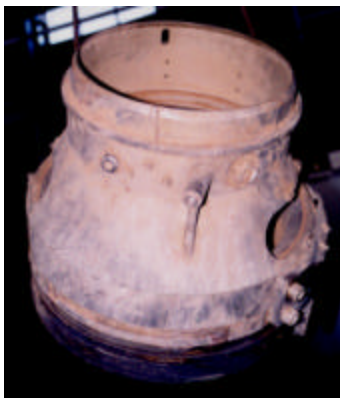
Fig. 33 (left). Terrier – Orion adaptor showing the abrasion damage over the external surfaces produced during ground impact.
