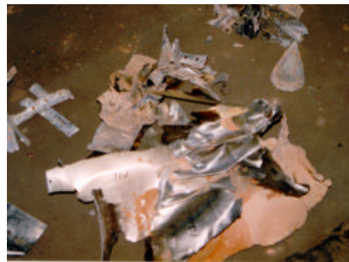
Fig. 8 (top L). Debris and remnants of the HyShot scramjet payload and Orion motor casing.
