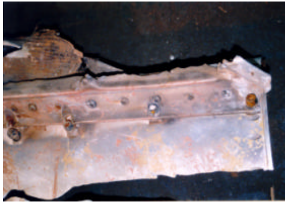
Figs. 31 (left) & 32 (above). Failure of the surface skin from the missing fin. Note the differences between the heavily heated side (above) and the opposite side (left).
