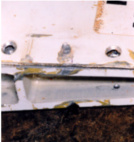
Fig. 53 (left). Clamping point for the fin securing lug – note the disruption produced by in-flight movement.
