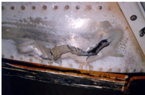
Fig. 21. Closer view of the burn-through area shown in figure 16.
