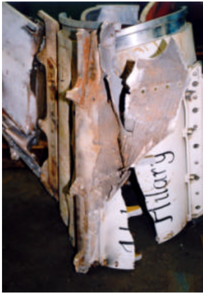
Figs. 31 (left) & 32 (above). Failure of the surface skin from the missing fin. Note the differences between the heavily heated side (above) and the opposite side (left).
