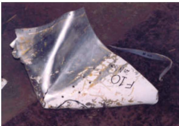
Fig. 51. Nike fin skin section, showing abrasion and removal of the paint from the leading face surface.
