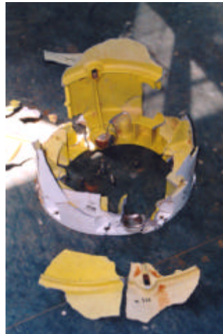
Fig. 42 (left). Terrier motor base with the remnants of the fin support structure in place.
