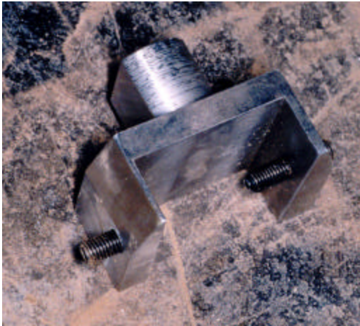
Fig. 5. Fin securing lug, as manufactured for the Terrier vehicle to suit the Nike fins.
