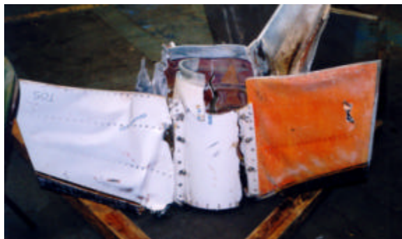
Fig. 18. Bands of heating behind the leading edge of an Orion fin.
