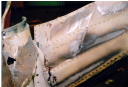
Fig. 28 (top left). Re-assembled tail can and fins, showing the orientation between the missing fin and the impact mark on an adjacent fin (arrowed).
