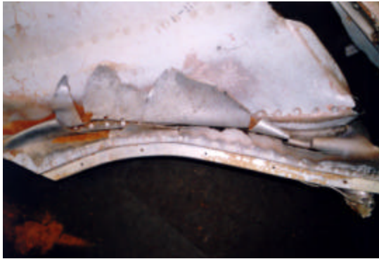
Fig. 23. Fin leading edge strip. Showing no thermal damage, despite the obvious damage to the skin behind.
