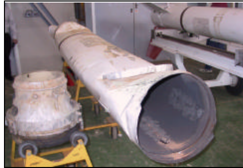
FIGURE 2. Recovered first stage alongside the adaptor and the assembled unused first stage.
