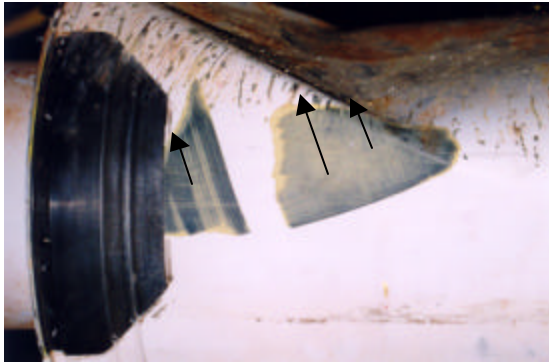
Fig. 40. Nike fin impact mark with the side of the Terrier motor casing. The direction of the impact is shown.
