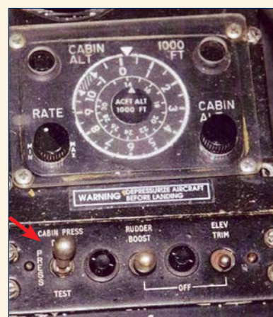
Typical King Air C90 cabin pressurisation controller with adjacent three-position cabin pressure control switch indicated by arrow
