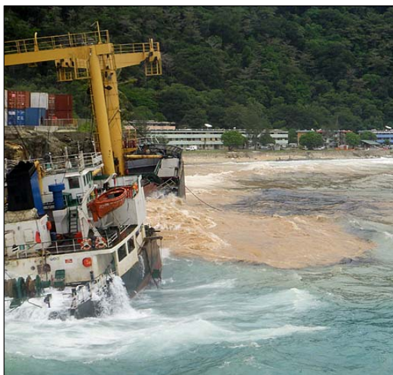
Figure 7: Failure of ship's hull at number 2 hold
