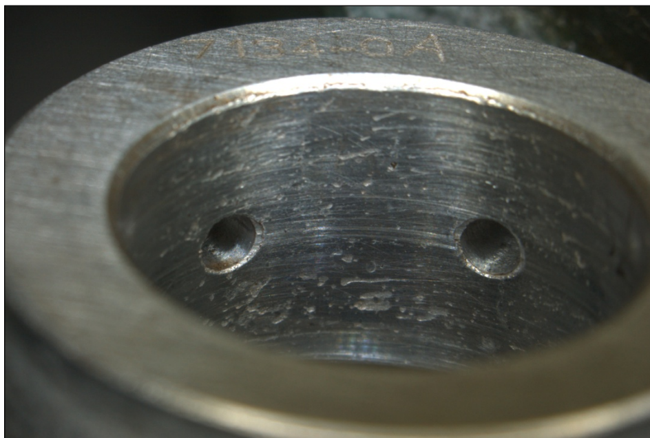
Figure 20: Internal surface of bearing showing scoring damage (YEO30243).
