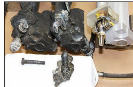
Left and right hydraulic boost servos
