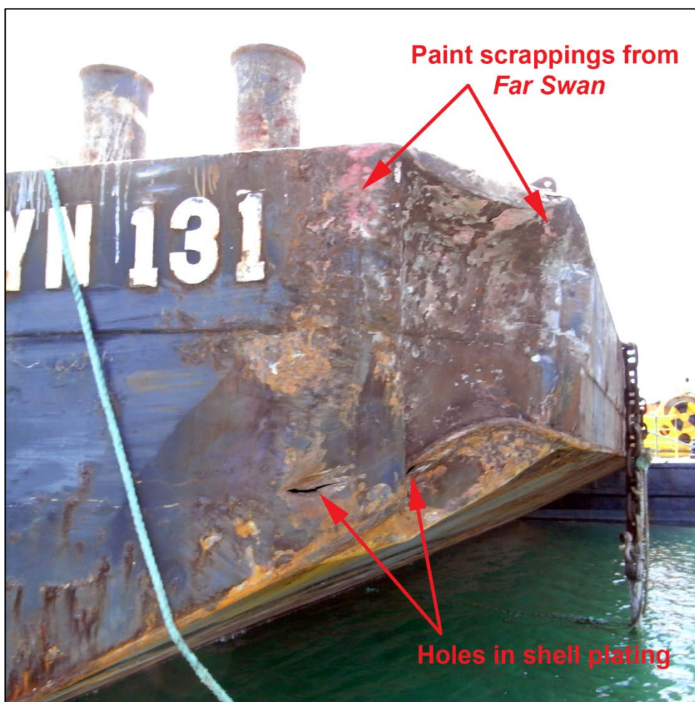
Figure 7: Damage to Miclyn 131
