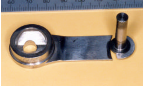
Fig. 2 Underside of the VSV lever removed from the engine.
