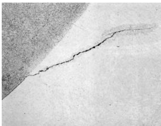
Fig. 8 (Left below) Closer view of the cracking shown in figure 7. Note the initiation from the end of a fused area around the pin circumference. Magnification X 115
