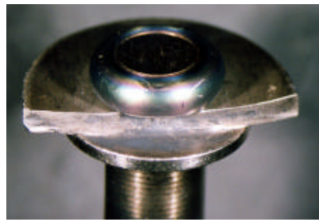
Fig. 5 Pin section fracture – adjoins the surface shown in figure 4.
