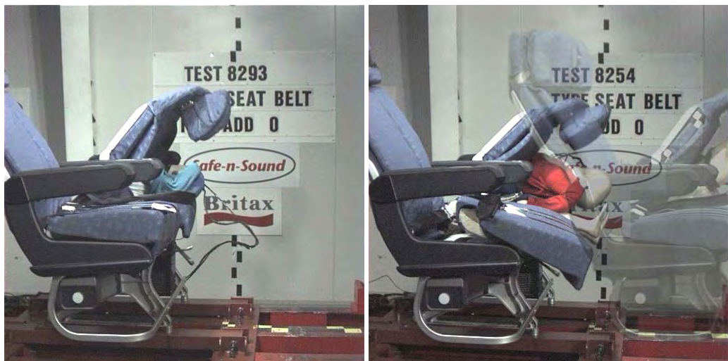
Figure 2.20. TNO P3/4 (9 kg) dummy (left) and TNO P3 (15 kg) dummy (right) in aircraft lap belt only
