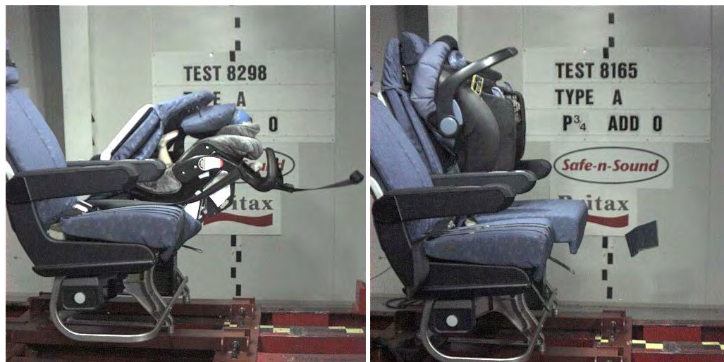
Figure 2.15. Rearward-facing infant restraints in sled tests showing (left) excessive forward flexion of the aircraft seat back, and (right) excessive rotation of the restraint about the lap belt upon rebound
