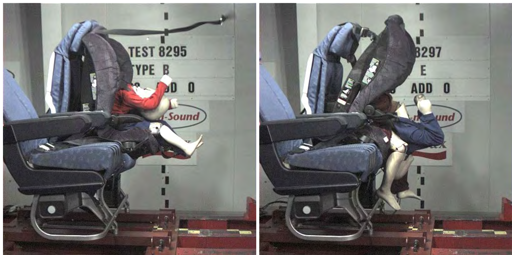
Figure 2.18. 2005 Model Safe-n-Sound Maxi Rider as a child restraint with harness and Qantas top tether (left), and a booster seat with aircraft lap belt and Qantas top tether (right)
