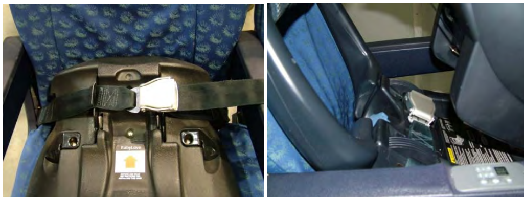
Figure 2.4. Incompatibility of infant restraint base mounts with the aircraft seat lap belt
