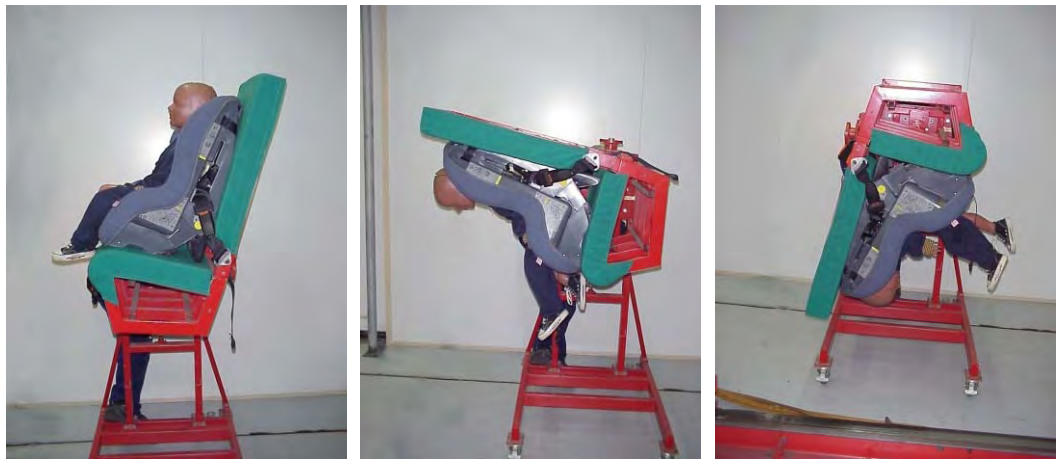
Figure 2.9. A TNO 3-year-old dummy in a Safe-n-Sound Royale CRS mounted in the aircraft style seat of the inversion test rig, undergoing the 180 degrees forward rotation
