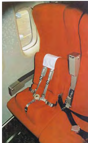
Figure 1.1. The AFI CareChair provided by Virgin-Atlantic is CAA approved since 1992 for use by infants from 6 months to 3 years of age (Gooding 1999)
