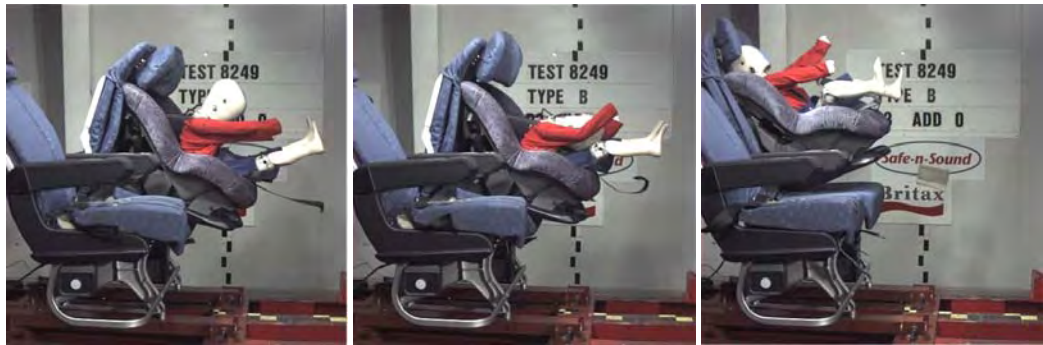
Figure 2.16. Motion of the TNO P3 (15 kg) dummy in the Safe-n-Sound Discovery type B CRS
