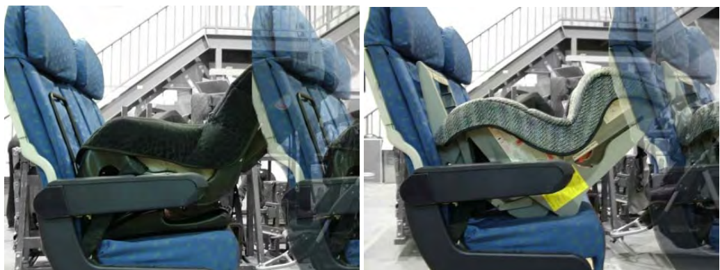
Figure 2.6. Superimposed images to show the fit of convertible child restraints in reclined rearward-facing mode within a 31-inch aircraft seat pitch
