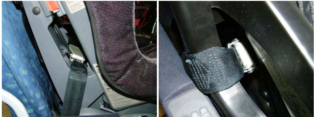
Figure 2.7. Access problems in engagement, adjustment and release of aircraft lap belt latch
