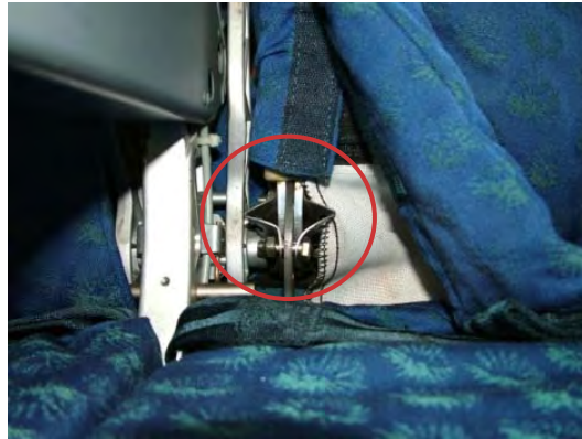
Figure 3.1. Damage to the forward seat back hinge
