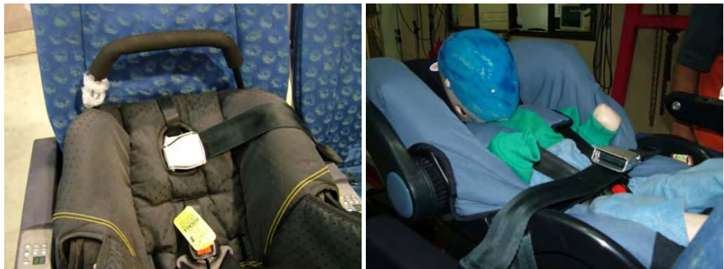
Figure 2.5. Location of the aircraft lap belt latch for rearward-facing restraints without a base mount: a) under the infant (left) or b) over the infant (right)
