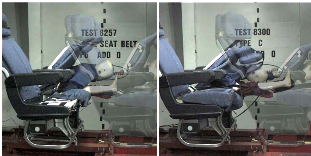
Figure 2.21. TNO P6 (22 kg) dummy in aircraft lap belt only (left) and in the lap belt with harness and Qantas top tether (right)
