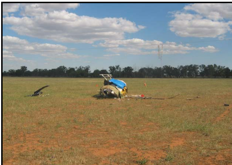
Figure 1: Bell 206B helicopter after striking powerlines during a locust control campaign near Forbes on 31 October 2004
