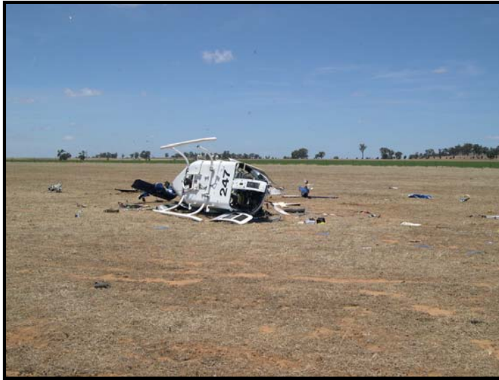
Figure 2: Bell 206B helicopter after striking powerlines during a locust control campaign near Dunedoo on 22 November 2004
