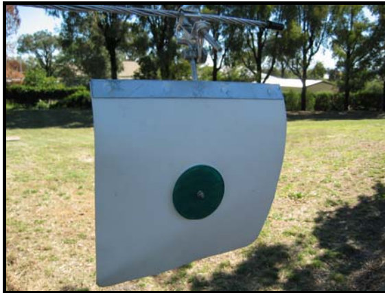
Figure 16: Example of a ‘flag marker’ used for aerial operations
