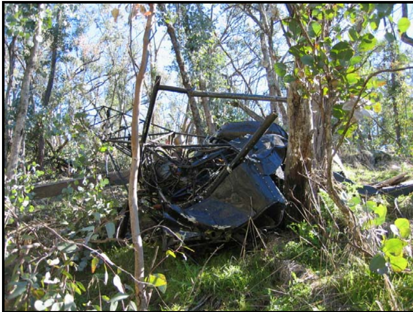
Figure 7: Bell 47G-3B-1 Soloy helicopter after striking powerlines near Wodonga on 19 June 2004
