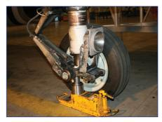
Boeing's recommendations come as a result of an ATSB investigation into a 25 July 2009 occurrence where a Boeing 737 lost a nose wheel tyre while taxiing towards the runway at Melbourne Airport. The right wheel detached from the nose landing gear due to an axle fracture.
