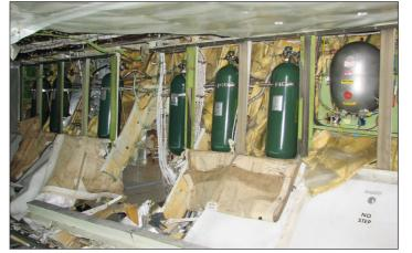
'We then identified five key hypothetical scenarios or possibilities on how the cylinder could have been damaged. These included: the cylinder having a manufacturing flaw; the cylinder being damaged before the last overhaul; the cylinder being damaged during the last overhaul; the cylinder being damaged after the last overhaul; the cylinder having been damaged during the accident flight.'
