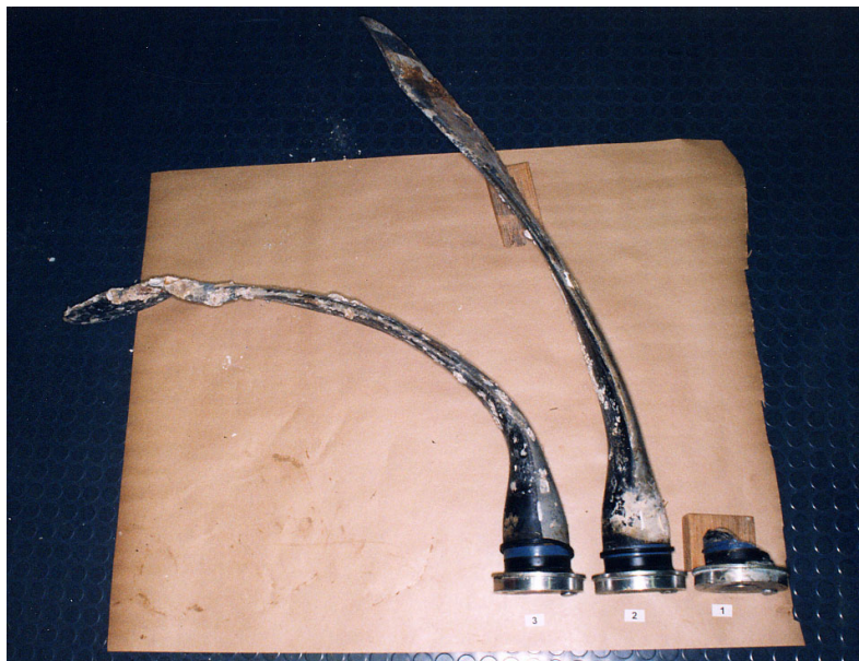
Figure 18. A Comparison of the extent of bending, with all blades in the same axial orientation. The failed blade probably sustained the greatest level of bending and fractured as a result.
