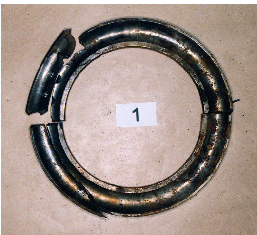
Figure 13. Thrust bearing race from the fractured blade. The crushing damage was found on the forward-facing side.
