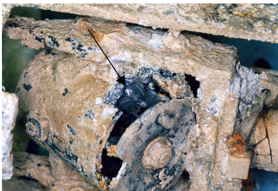
Figure 4. Gyro housing, showing the fragment of instrument glass inside
