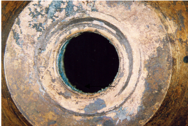
Figure 8. Gyro rotor end face, also showing evidence of rotational scoring.
