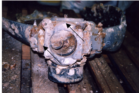
Figure 12. Blade fracture surfaces, giving some indication of the direction of failure.
