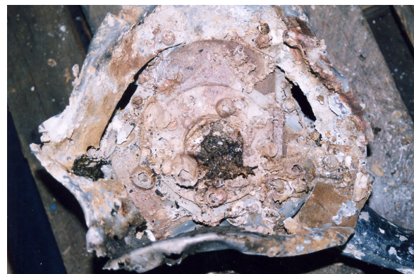
Figure 10. Level of marine growth and accretions typically present over the entire unit.
