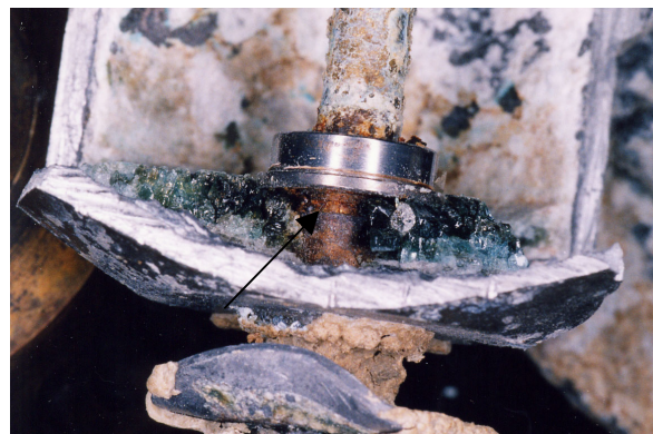
Figure 5. Gyro housing, showing forward movement of the inner bearing.
