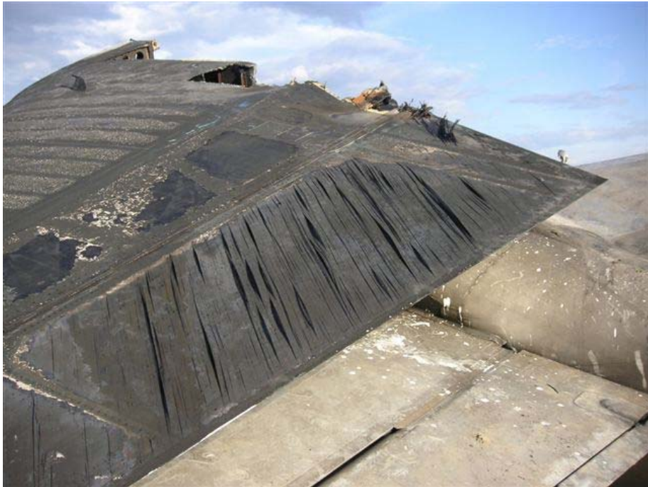
Figure 13: Burnt composite fibres in the rudder section of a Boeing 737-400 following a post-impact fire
