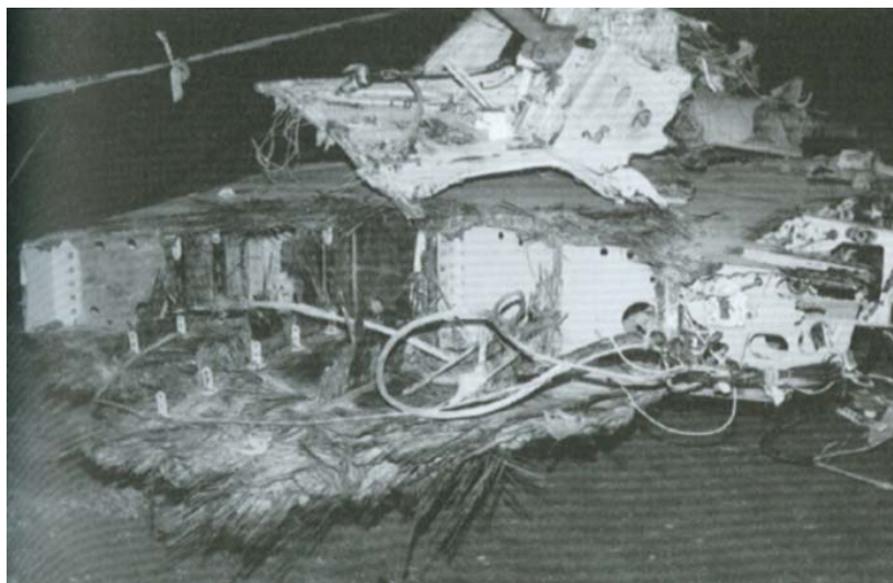
Figure 10: Wing that failed in bending, showing the difference between the tension (lower) and compression (upper) sides
