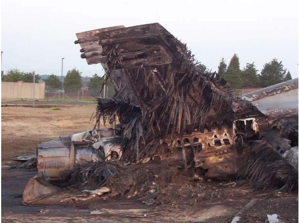
Figure 15: Significant carbon fibre debris following an F/A-18 Hornet fire – a typical scene at future accident sites?
