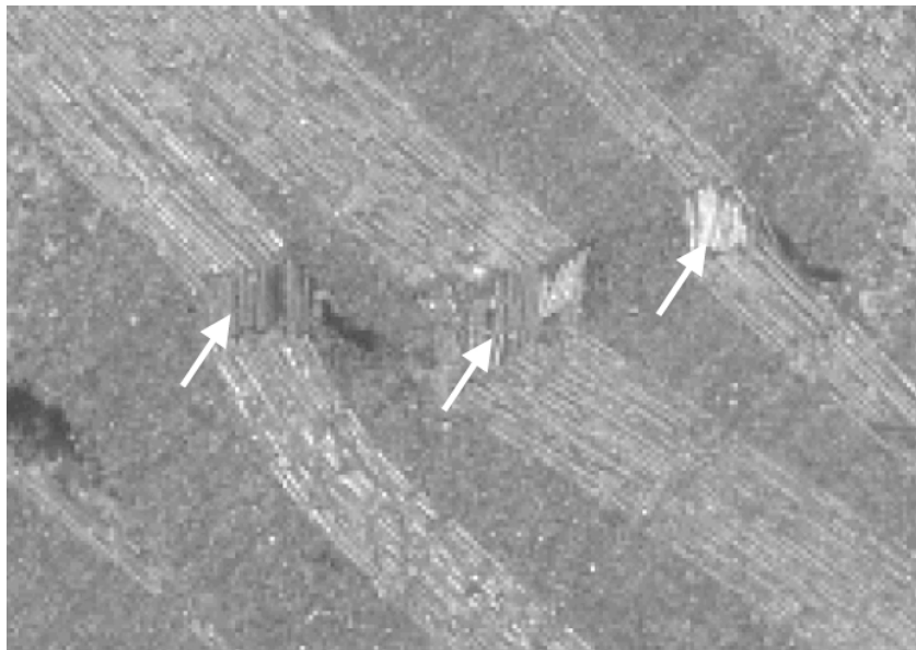
Figure 8: Formation of kink bands when composite laminates are under compression (marked with arrows)
