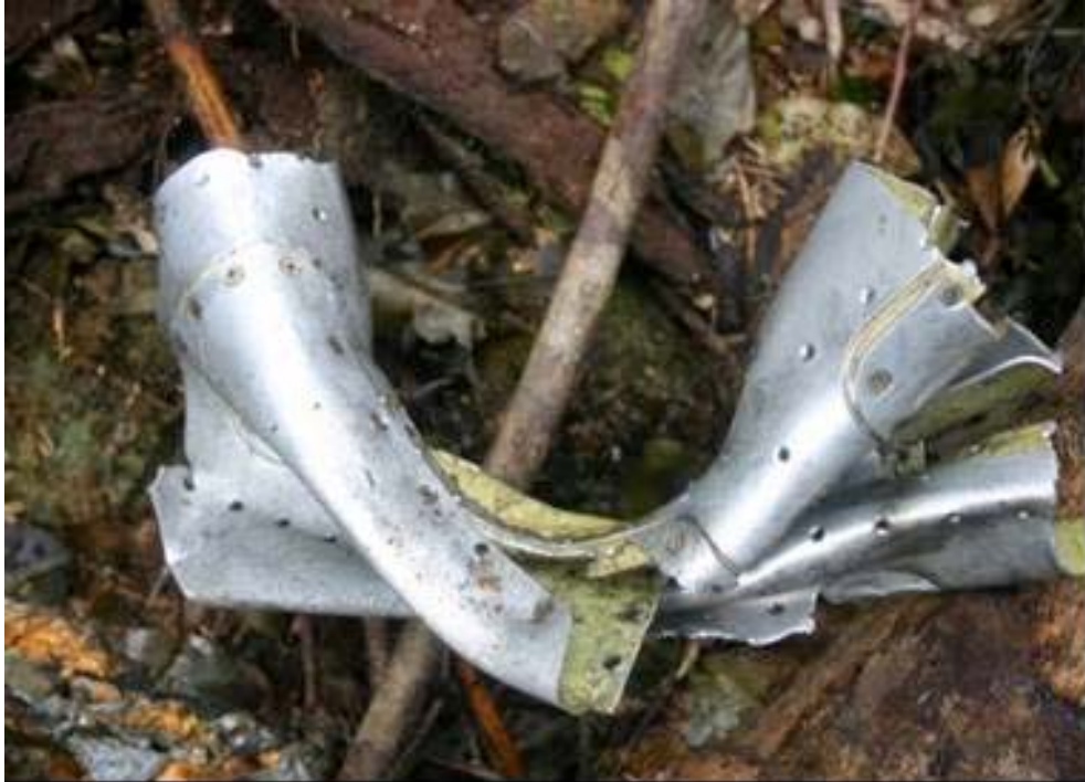
Figure 15: Wing section showing impact damage with a tree trunk or branch
