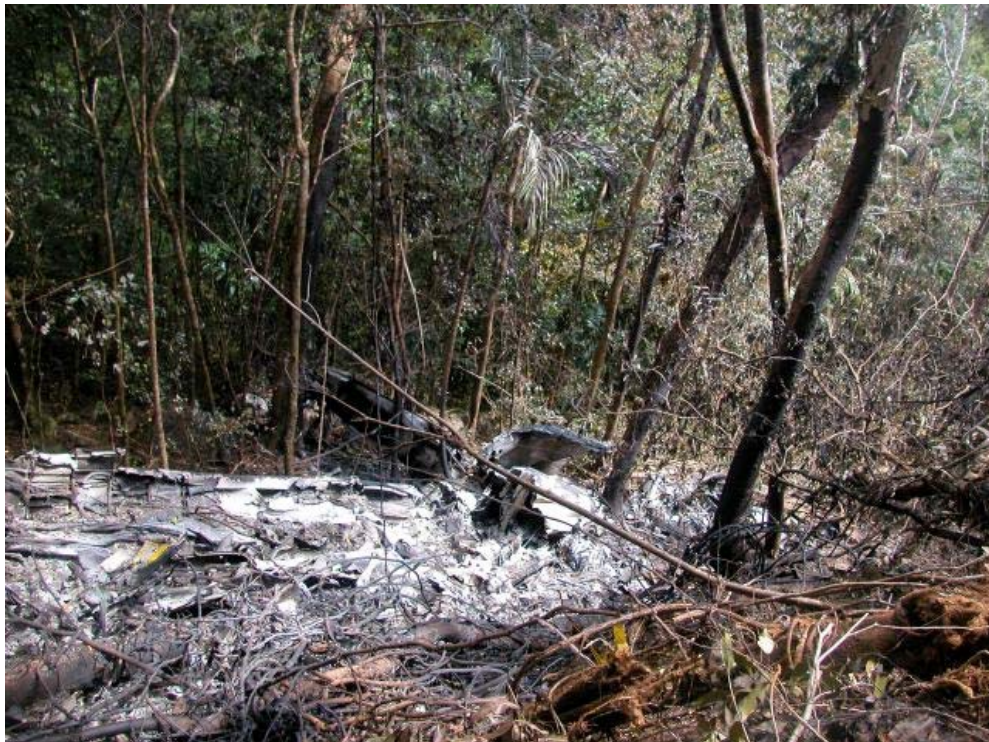
Figure 17: The rear fuselage section
