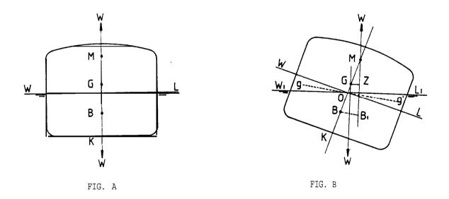
If the ship is inclined by an external force to a small angle as shown in Figure B the centre of gravity will remain at G and the weight of the ship (W) can be considered to act vertically downwards through this point. The centre of buoyancy shifts from B to B1
