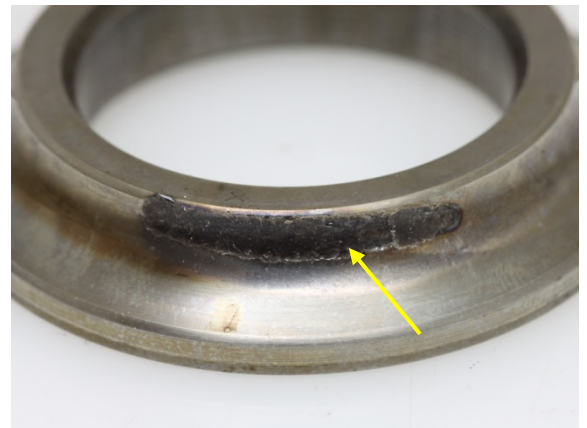
Figure 4: Number-1 bearing inner race showing electrical discharge damage
