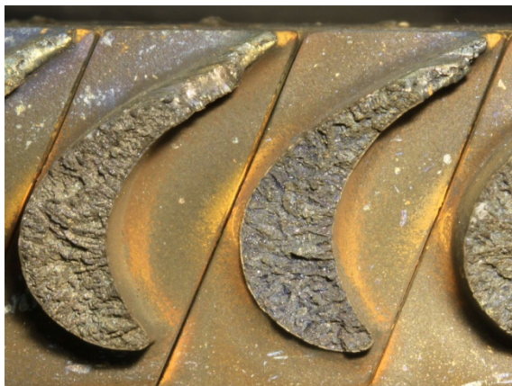
Figure 3: Typical CT blade fracture surfaces
