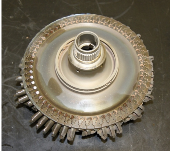
Figure 3: Typical CT blade fracture surfaces
