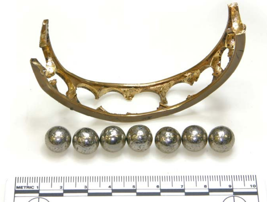
Figure 9: The fragmented cage and some of the bearing balls as-recovered from the mast bearing assembly
