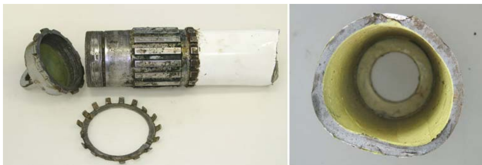
Figure 4: The detached mast cover nut (left) and fractured upper portion of the main rotor mast (right)
