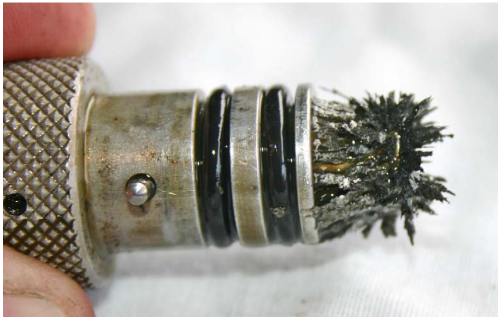
Figure 7: The magnetic drain plug showing metallic particles amassed around the tip
