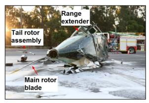
The fuel tank was punctured by the skid-landing gear rear crosstube, which was driven up through the fuselage by vertical deceleration forces. The main rotor blades were slightly damaged. Examination of the wreckage confirmed that all of the damage was the result of impact forces.
