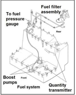
There was a non-return valve between each electric fuel boost pump and the engine. In the event that the inlet to an electric fuel boost pump was no longer covered by fuel, or if a pump ceased to operate, its non-return valve would be closed by the fuel pressure from the other pump. That ensured that fuel would not be pumped back into the tank, that the fuel supply to the engine would continue, and the FUEL PUMP warning light would illuminate.
