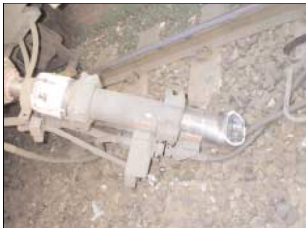
FIGURE 4: Collapsed as designed Scharfenberg coupler
