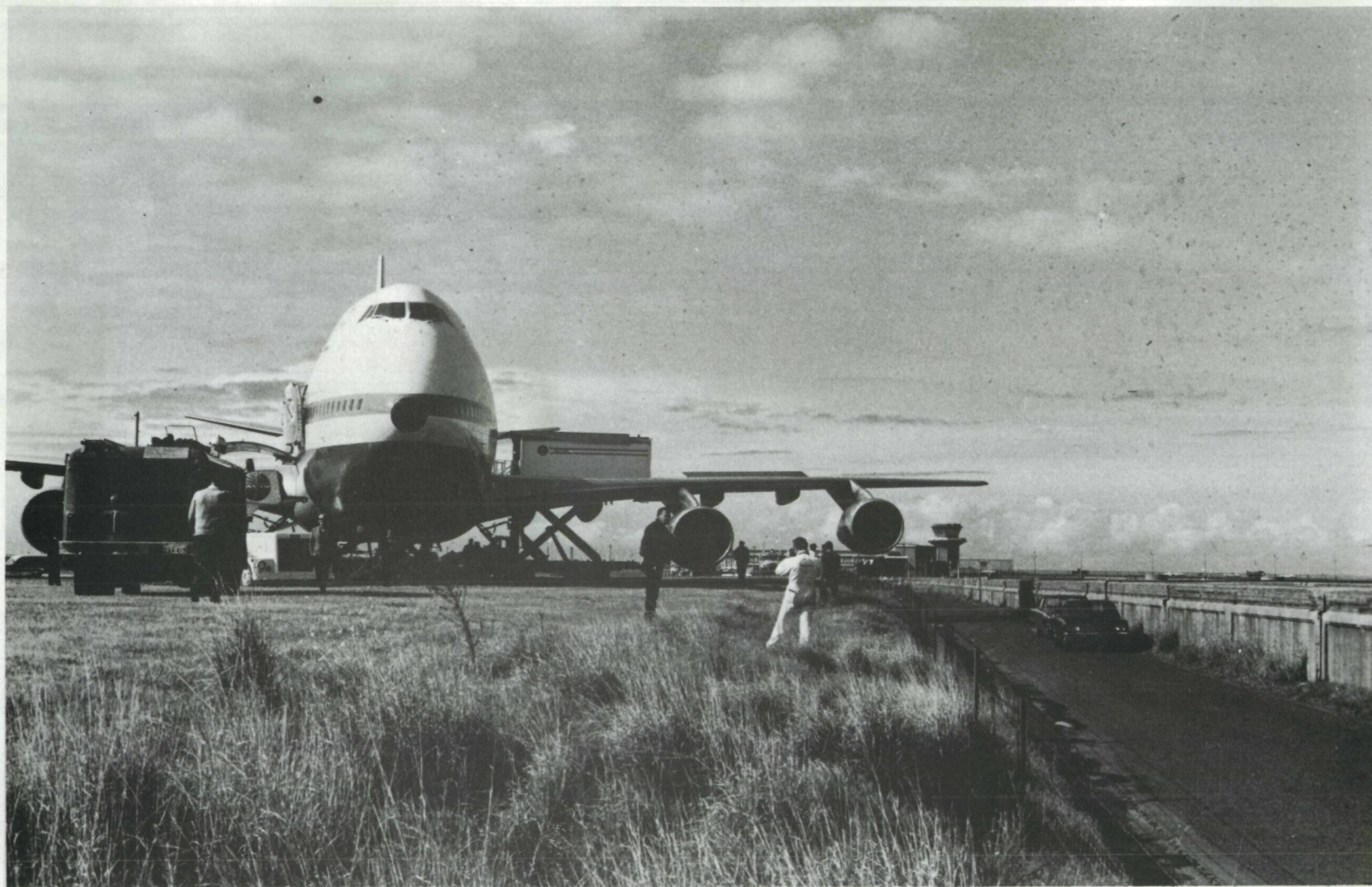
The aircraft as it came to rest a short distance beyond the end of the runway. Note the sunken perimeter road and the sewage outfall.
