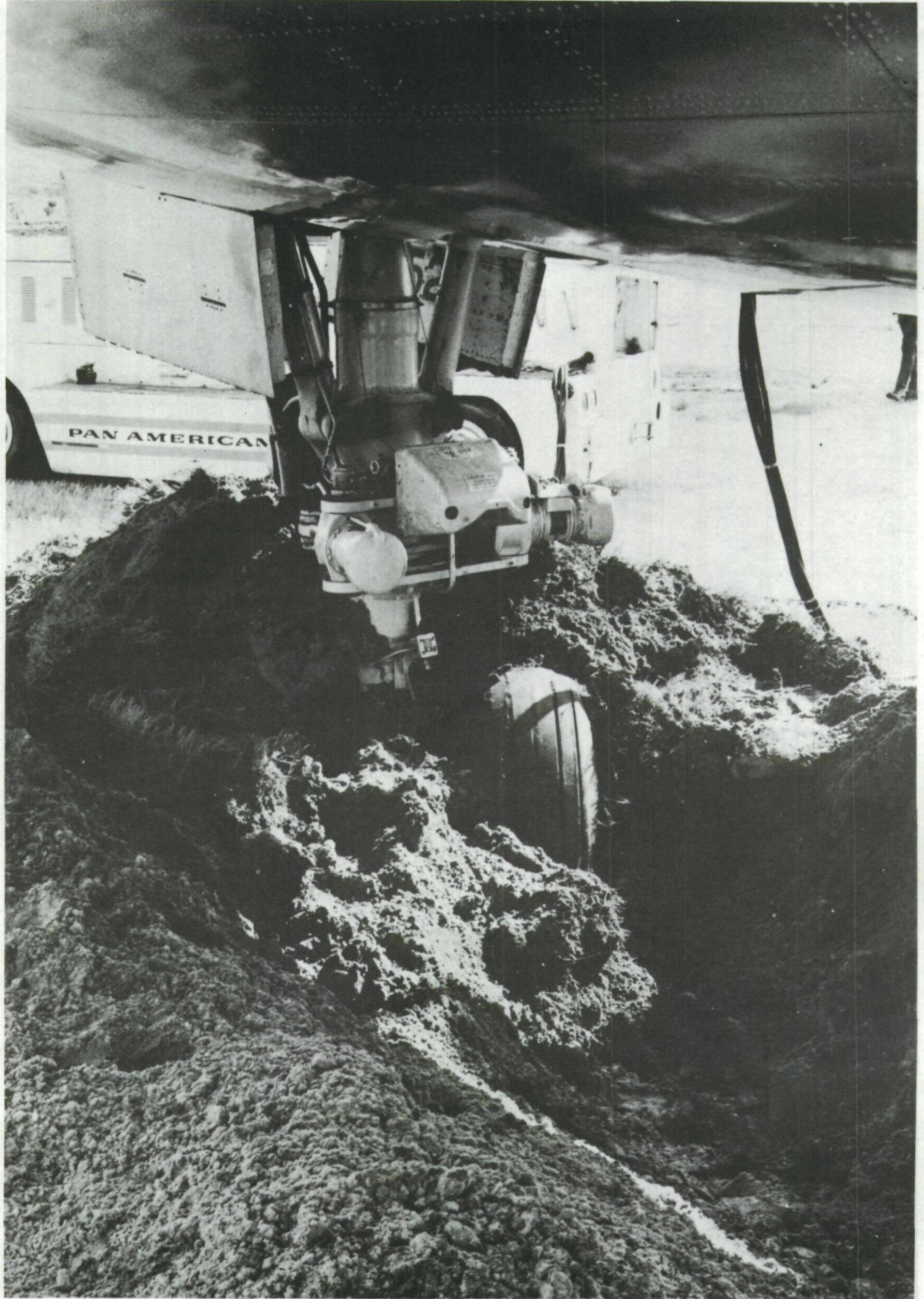
The nose undercarriage of N652PA showing the depth to which the wheels penetrated the soft earth.
