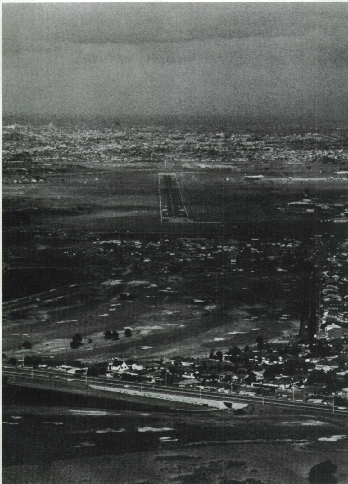
Runway 25 as seen from a position on a three degree approach slope, approximately two miles from the landing threshold.
