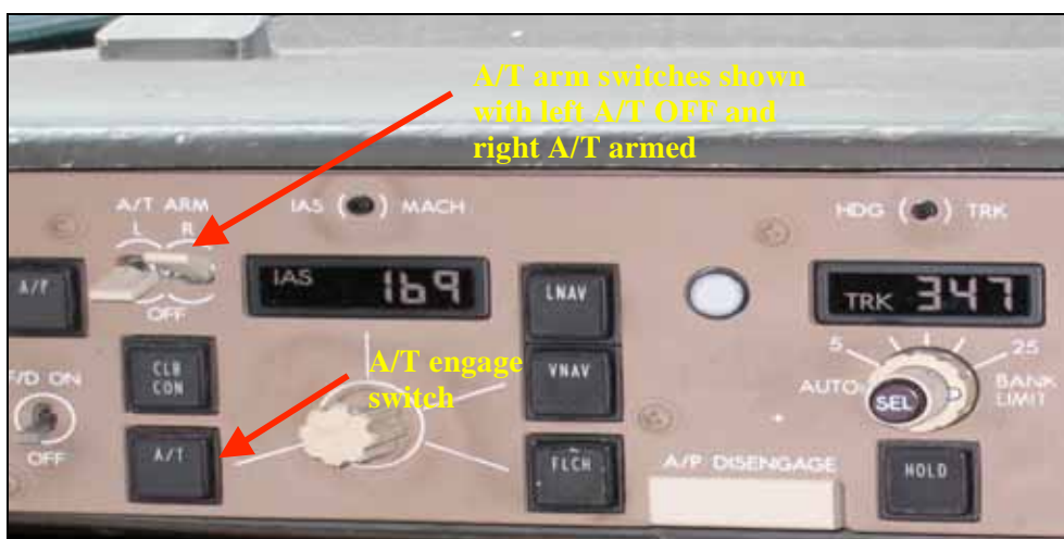
Figure 4: MCP autothrottle arm and engage switches
