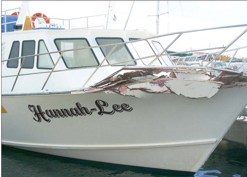
FIGURE 4: Hannah Lee damage to starboard bow
