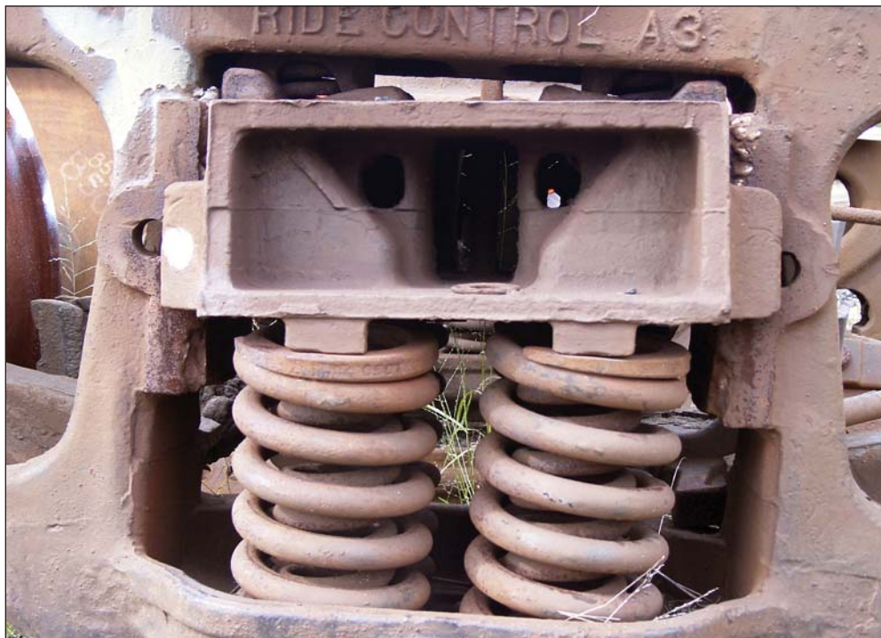
FIGURE 13: Typical bogie spring nest showing inner and outer springs
