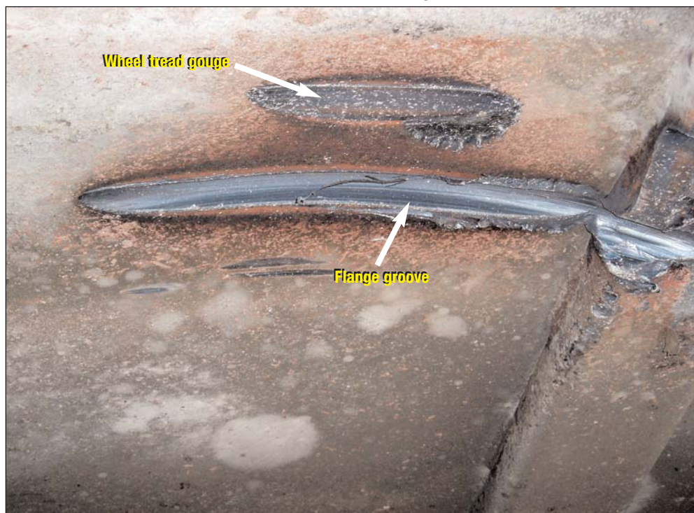
FIGURE 9: Indent marks underside of VQCY from wheel flange
