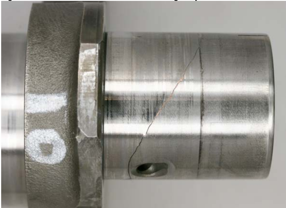
Figure 4: Crack in the number one connecting rod journal.
