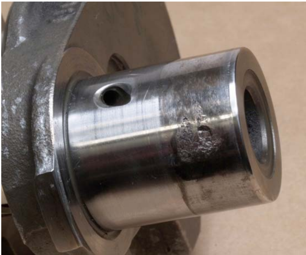
Figure 8: Adhesive wear on number two connecting rod journal.
