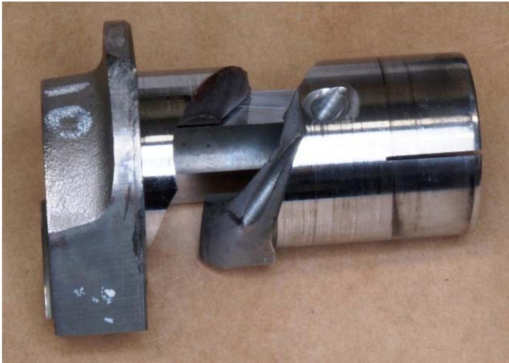
Figure 11: Failed number one connecting rod journal.
