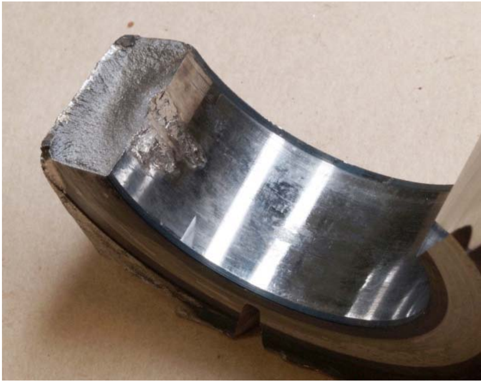
Figure 7: Failure 'B' in crank web with adhesive wear on journal contact surface.
