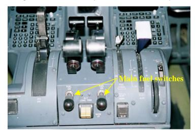
Figure 1: Boeing 717 throttle module (fuel switches indicated)
