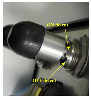
Figure 3: Fuel switch in an out of detent (unlocked), ON position
