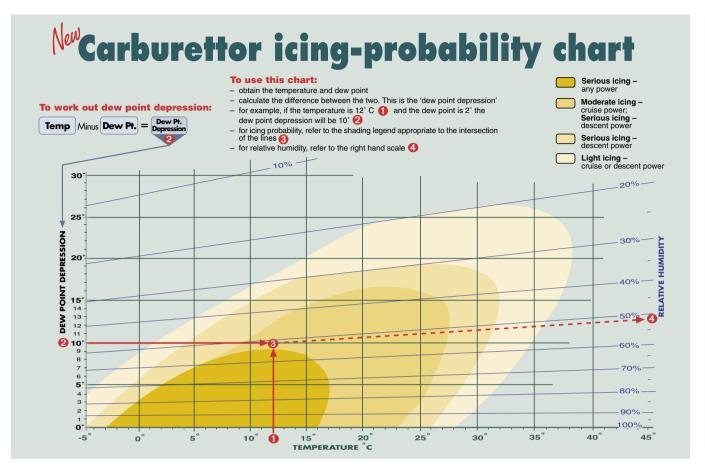
carburettor heat with throttle closure and check the engine's response to throttle movement frequently – on passing each 1,000 ft in a descent, for example.
