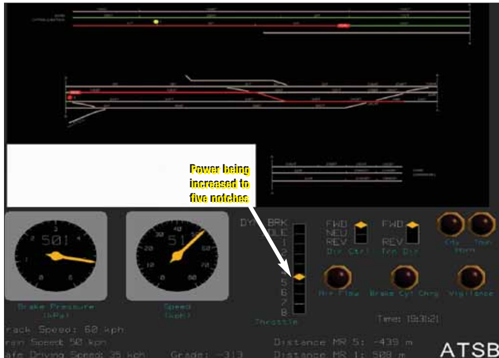
FIGURE 9: 1931:21 train Y245 439 metres from signal MR5, power being increased to five notches
