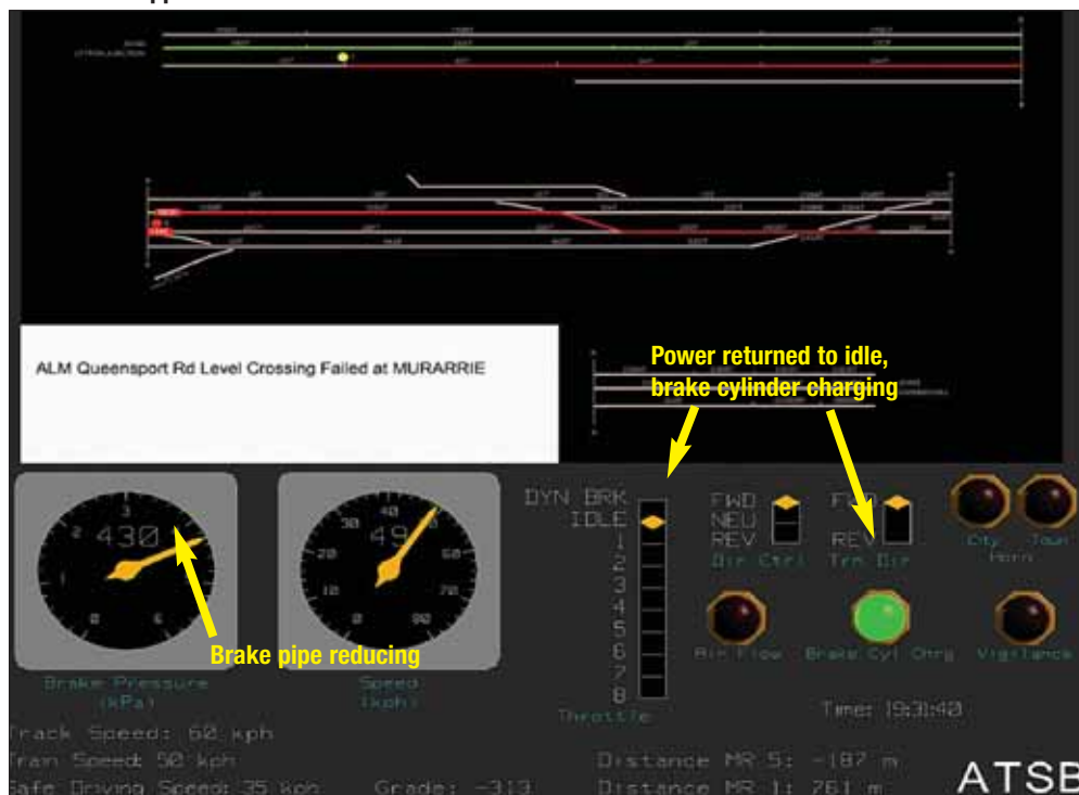
FIGURE 11: 1931:40, brake application initiated, UTC Queensport Road level crossing alarm first appears
