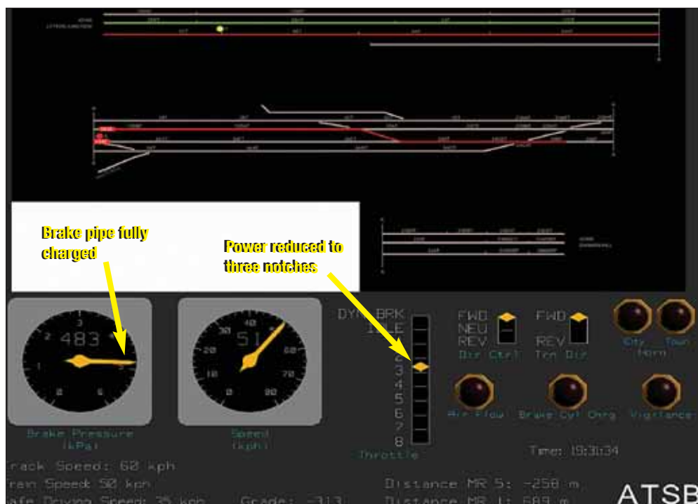
FIGURE 10: 1931:34, train Y245 at sighting distance (258 metres) from signal MR5
