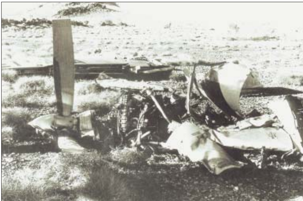
FIGURE 13: No. 4 engine and wing wreckage of Vickers Viscount VH-RMQ
