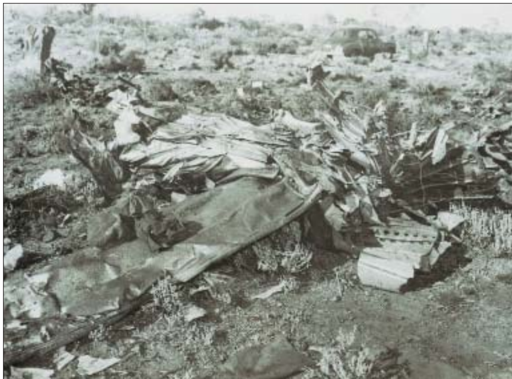
FIGURE 12: Rear fuselage and empennage of de Havilland Dove VH-AQO
