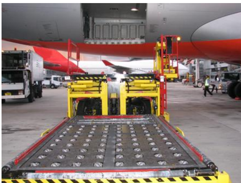
Figure 10: Pallet loader positioned next to an aircraft at an Australian airport
