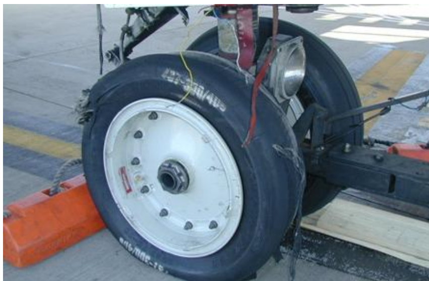
Figure 23: A Boeing 737 nosewheel tyre shredded as a result of FOD impact in Australia
