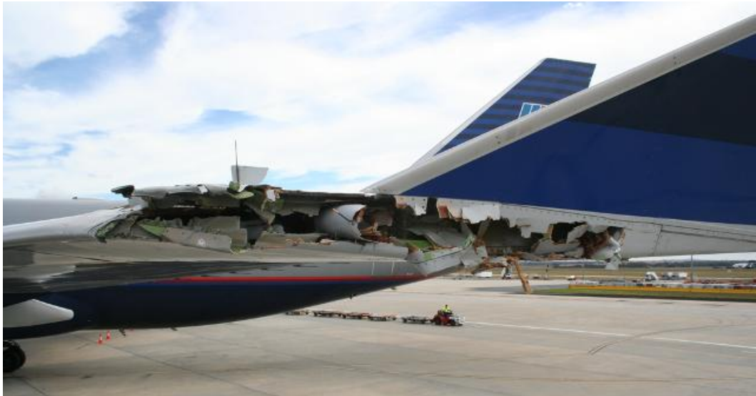
Figure 18: Taxiway aircraft-aircraft collision showing winglet damage
