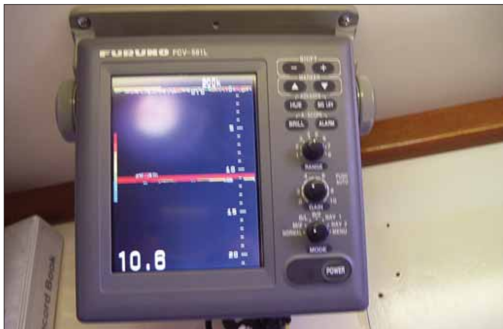
Figure 18: Echo sounder on board Leeuwin II
