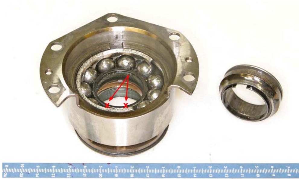
Figure 4: The compressor bearing as recovered from the right engine showing the major area of damage (arrowed)
