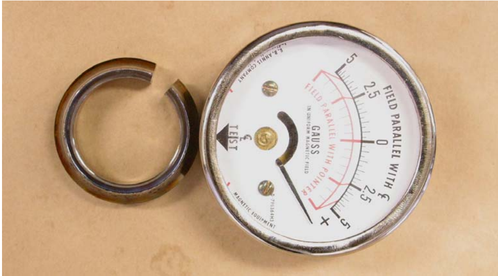
Figure 5: Inner race magnetisation as measured with a Gauss meter
