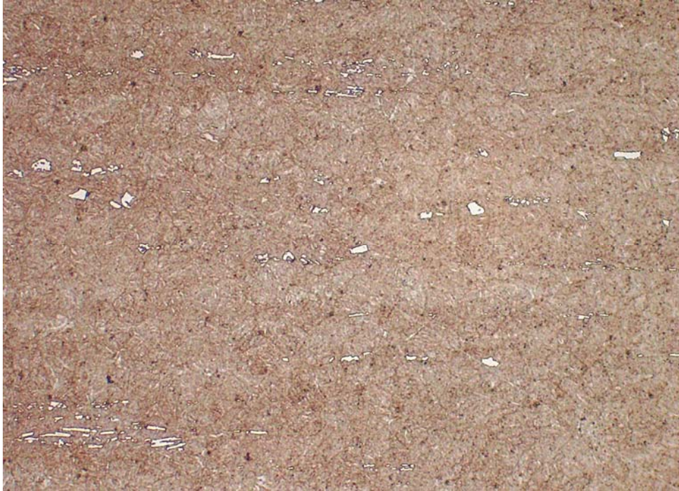
Figure 12: Section through a bearing ball showing the least heat affected microstructure
