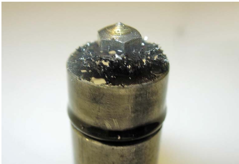
Figure 2: A picture of the reduction gearbox chip detector with metal particles clearly visible
