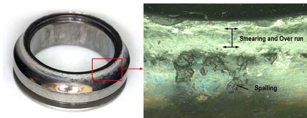
Figure 11: Image montage of the inner race puller-groove raceway surfaces showing over run and spalling damage
