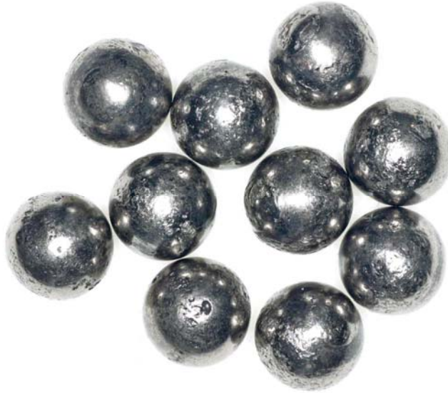
Figure 8: The rolling surface of each bearing ball had spalled
