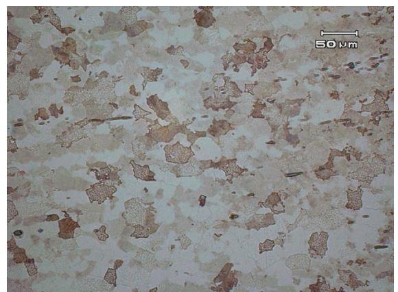
Figure 5: Steel microstructure (2% nital etch)
