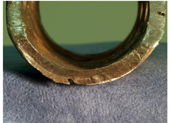
Figure 4: Remaining portion of weld
