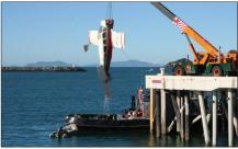
The aircraft decelerated rapidly and came to rest, floating in an upright position for about 1 minute. All of the occupants evacuated and were later recovered by a rescue helicopter. The engine power loss was consistent with fuel starvation. There had been insufficient time to resume power by selecting reserve fuel from such a low altitude before ditching.
