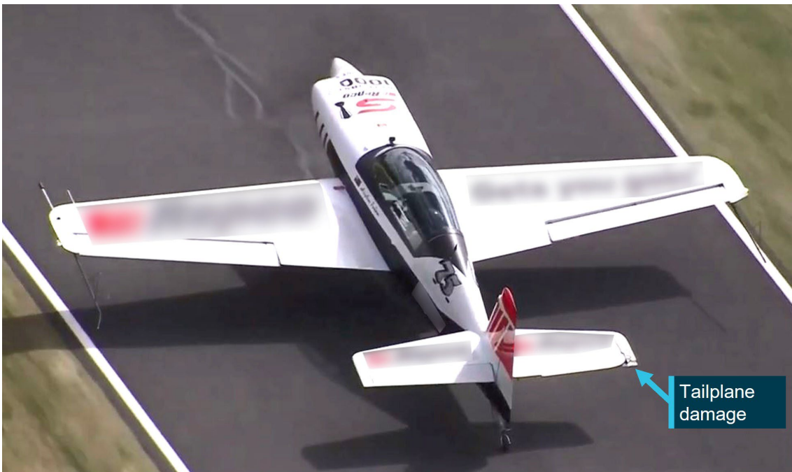
Figure 2: Tailplane damage after collision
