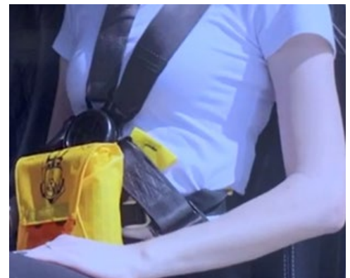
Incorrect fitment of seatbelt with constant wear lifejacket (source: Sea World Helicopters)
